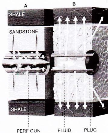
**PLUG AND PERFORATION** A plug blocks off a section of pipe, and a "perf gun" blasts small holes in the sandstone (A). Fluid is pumped in at high pressure (B), releasing the oil.
