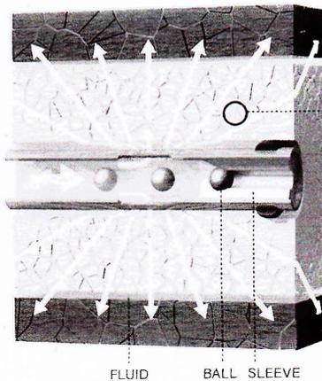
**SLIDING SLEEVE** Plastic balls are forced down the pipe, pushing open sliding sleeves to expose holes in the pipe. Fluid shoots out through the holes, fracturing the rock.
