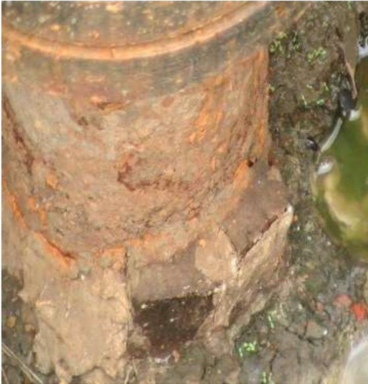
These 2 (two) are of Dewhurst 3c in the PEL 238 and clearly show that the outer casing at the top has been eaten away. This well is on Santos' plug and abandon list. My question is: If this is like this at the top where it can be seen, then what is the condition of the outer casing for the approx. 800 metres under the ground that cannot ever be seen once plugged with cement and can never be checked by any known method?
