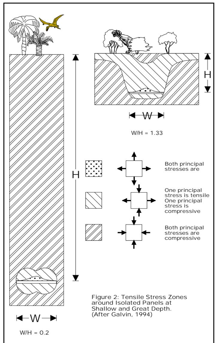
For this system to be successful the dimensions of coal pillars left must be sufficiently strong in order to accept the strata load previously carried by the mined coal from the void. In recent years the strength of pillars has been determined for Australian coals and can be expressed, for large pillars, by the form
