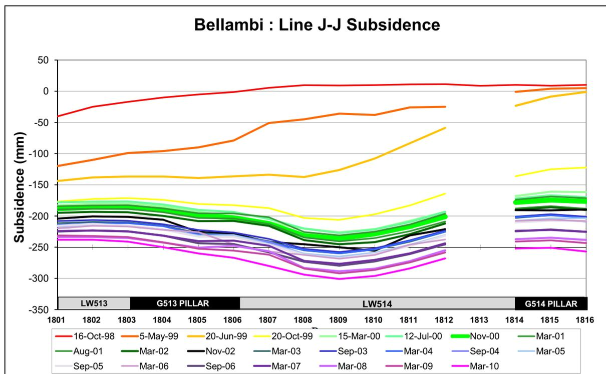
**Figure 12 Subsidence on J-J line with time**
