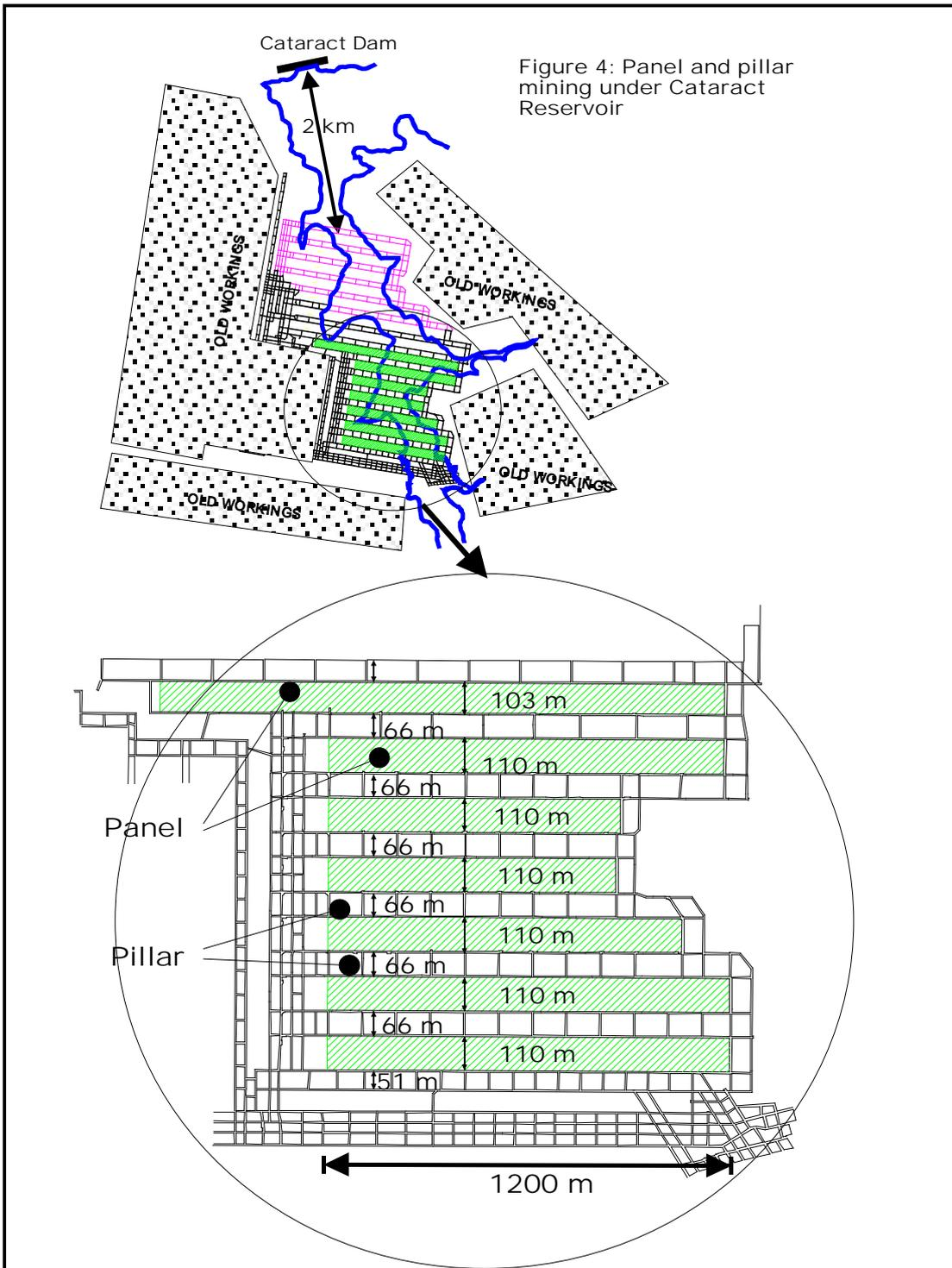
Figure 4: Panel and pillar mining under Cataract Reservoir
