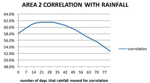
Figure 11 Area 2 correlation of rainfall with mine water balance by moving rainfall forward in time incrementally.
