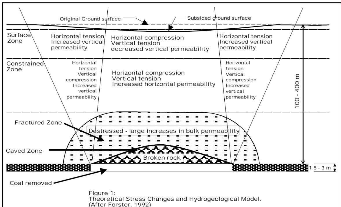
fracture the rock, although some localised fracturing would be expected. Here, it is believed that most large movements occur along horizontal planes between rock layers. This has been called the “constrained” zone because it is in this zone that barriers to vertical drainage are most likely to be found. However, the extent to which vertical permeability develops depends on whether impermeable layers exist before mining.
