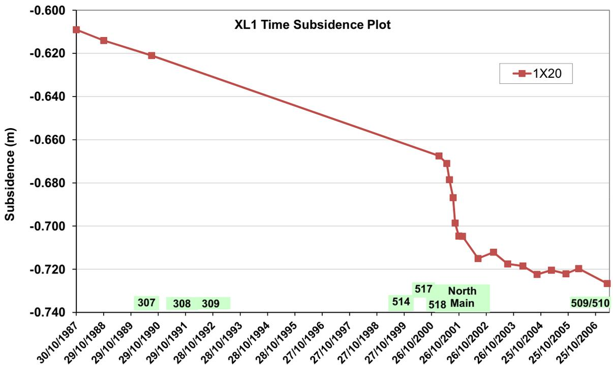
Figure 7 Time series of subsidence at Peg20 on Line XL1
