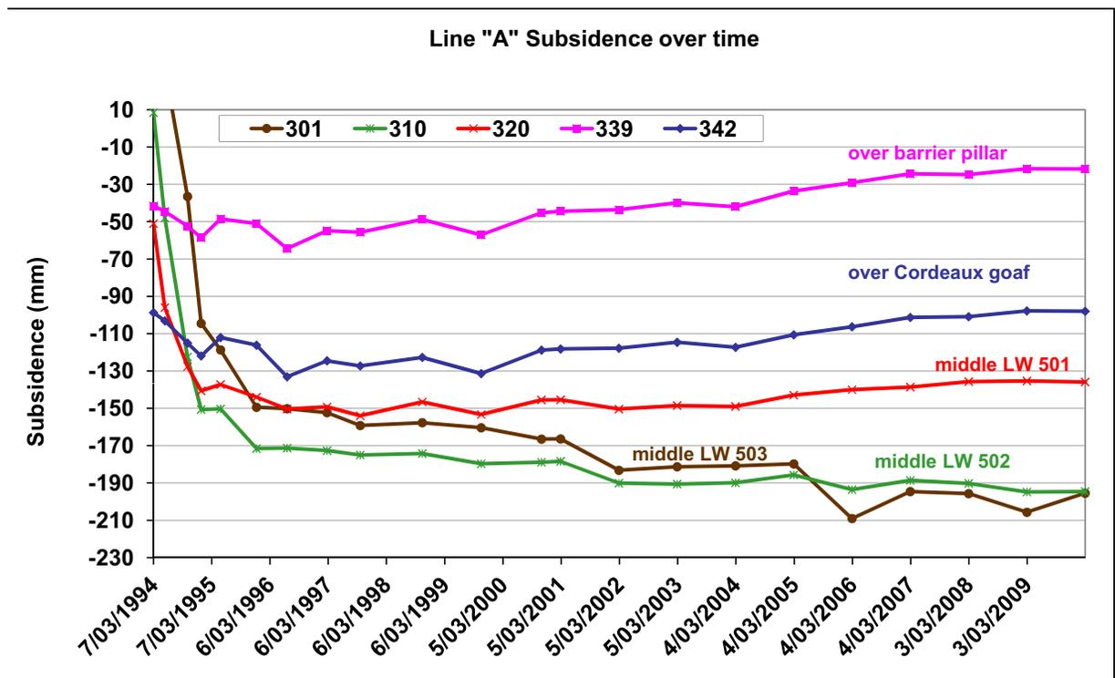
Figure 11 Time series of subsidence at various pegs along Line A-A
