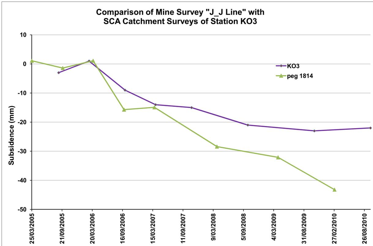
Figure 6 Comparison of Mine Survey 'J\_J Line' with SCA Catchment Surveys of Station KO3
