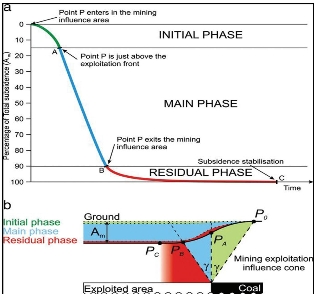
Figure 13 Residual subsidence (from Gueguen et al 2009)
