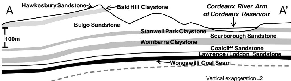
Figure 3 Cross section through Area 2 and Cordeaux River Arm of Cordeaux Reservoir (see location of cross section on Figure 1B).
