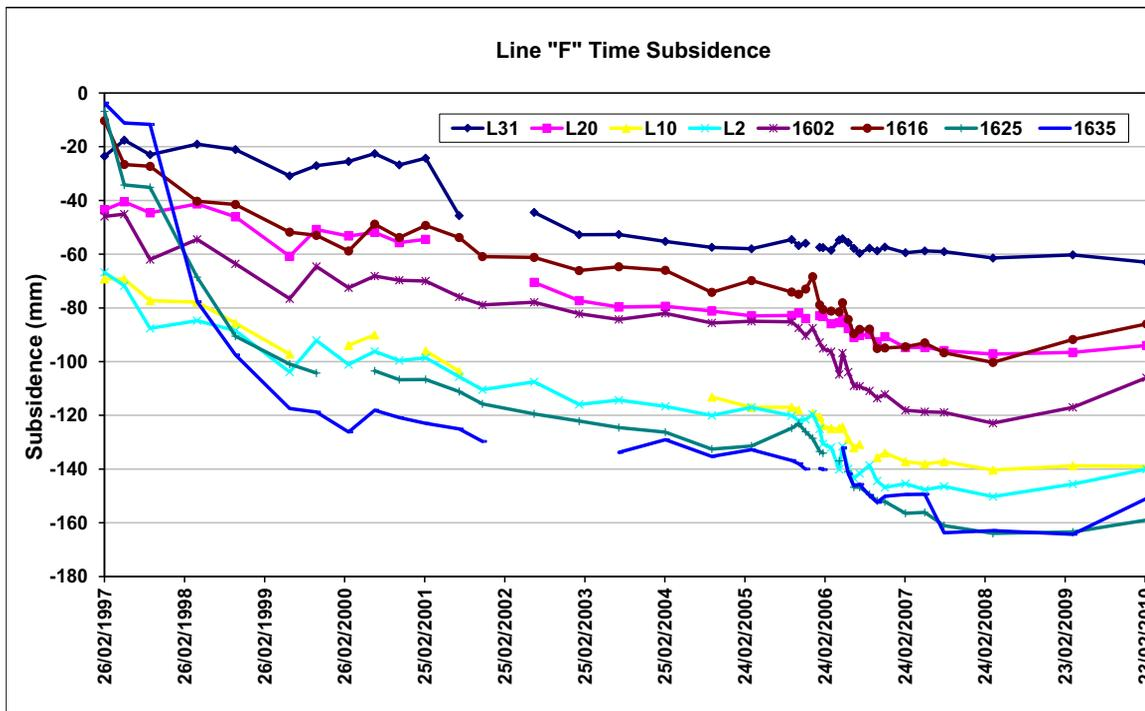
Figure 9 Time series of subsidence at various pegs along Line F-F
