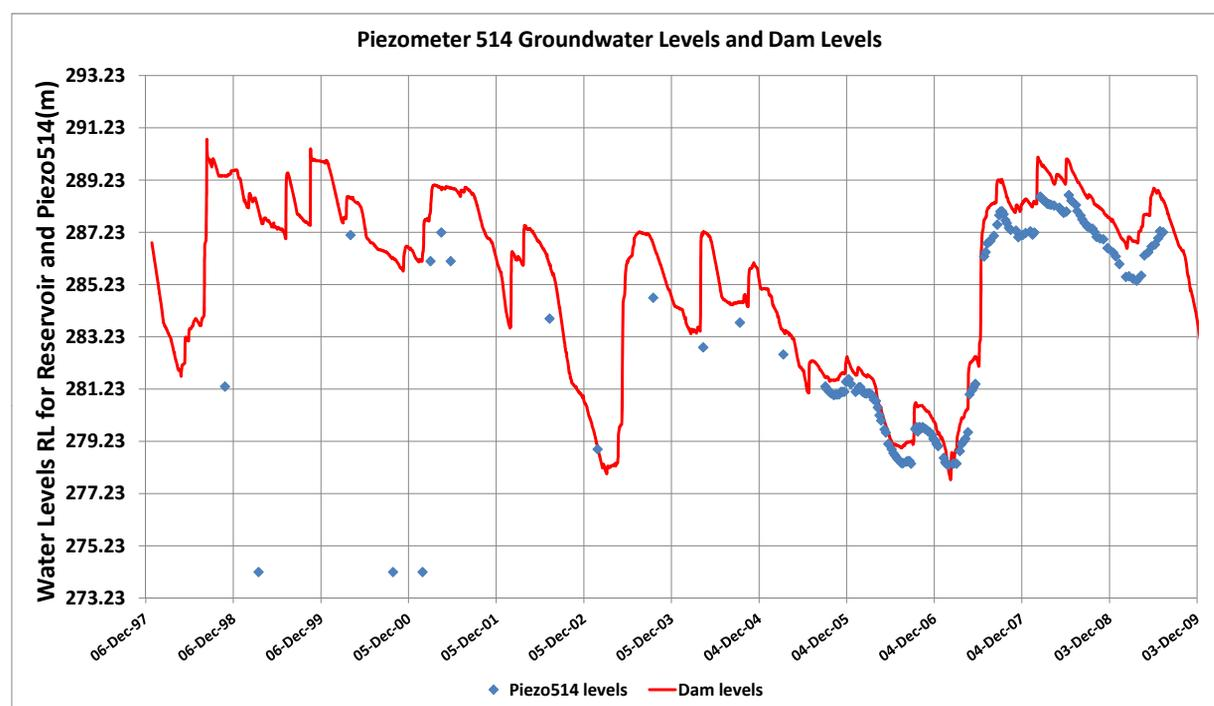
Figure 14 Comparison of groundwater and dam levels
