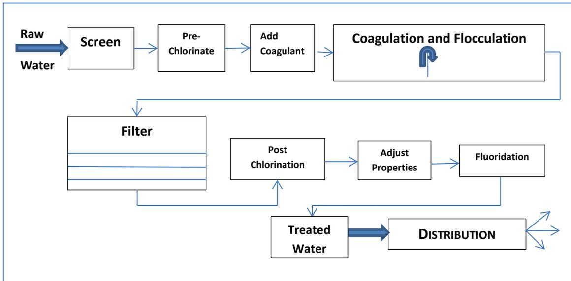
**Figure 3: Water Filtration Plant**
