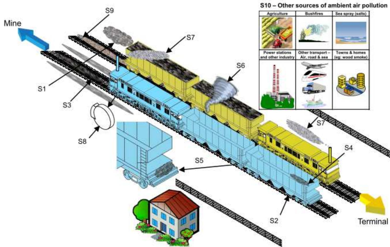
Figure 1: Potential sources of dust emissions and factors affecting emissions in the rail corridor
