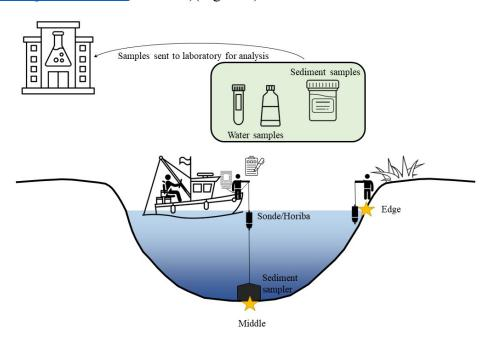
Figure 3. Schematic of middle and edge-sampling methodology including in-situ measurements (Sonde / Horiba) and water and sediment samples collected for laboratory analysis.
