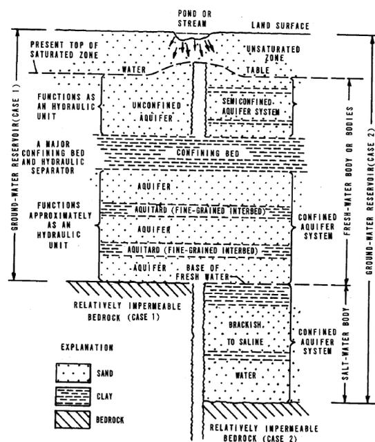
Figure 10. Schematic model for ground-water extraction (Poland, 1984)
