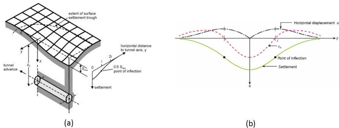
Figure 6. Tunnelling in soils. (a) Settlement trough (b) vertical and horizontal movements
