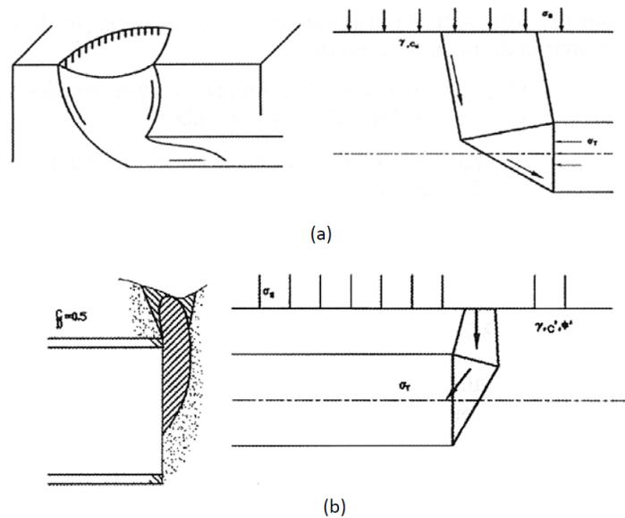
Figure 5. Face stability problems during tunnelling in soft ground (ITA-AITES, 2007)
