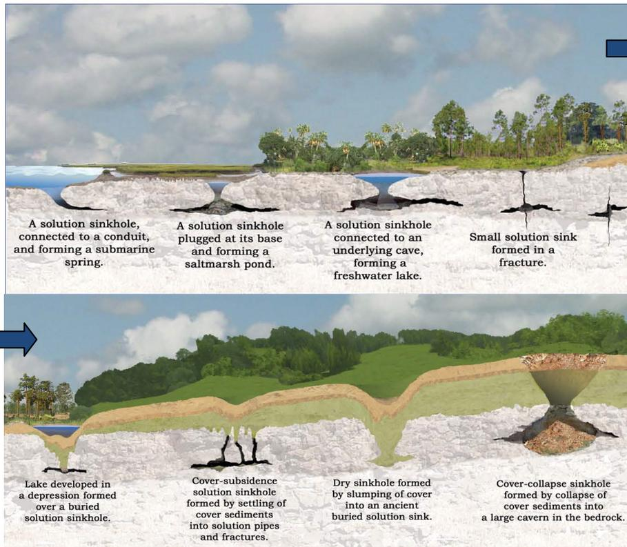
Figure 1. Types of sinkholes (modified from Rupert & Spencer, 2004)
