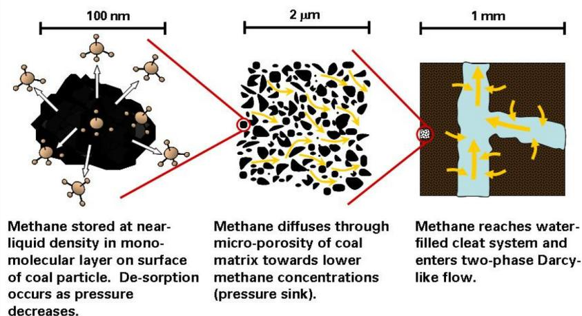
Figure 14. Movement of methane in coal (from Loftin, 2009).
