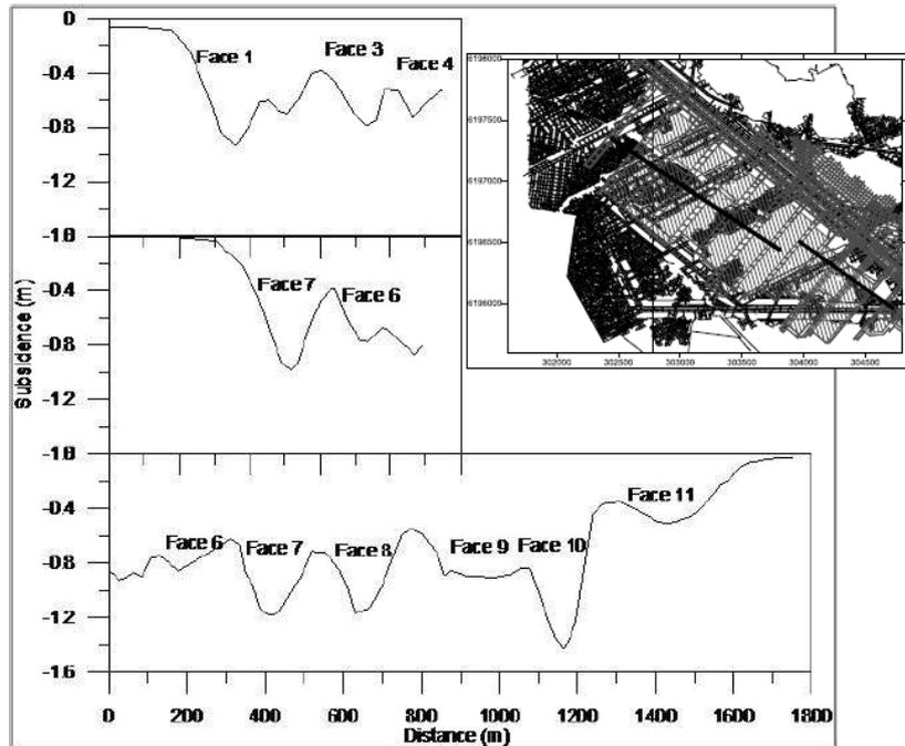
Figure 9. Subsidence registered in Balgownie seam longwall (from Seedsman Geotechnics Pty Ltd, 2011)
