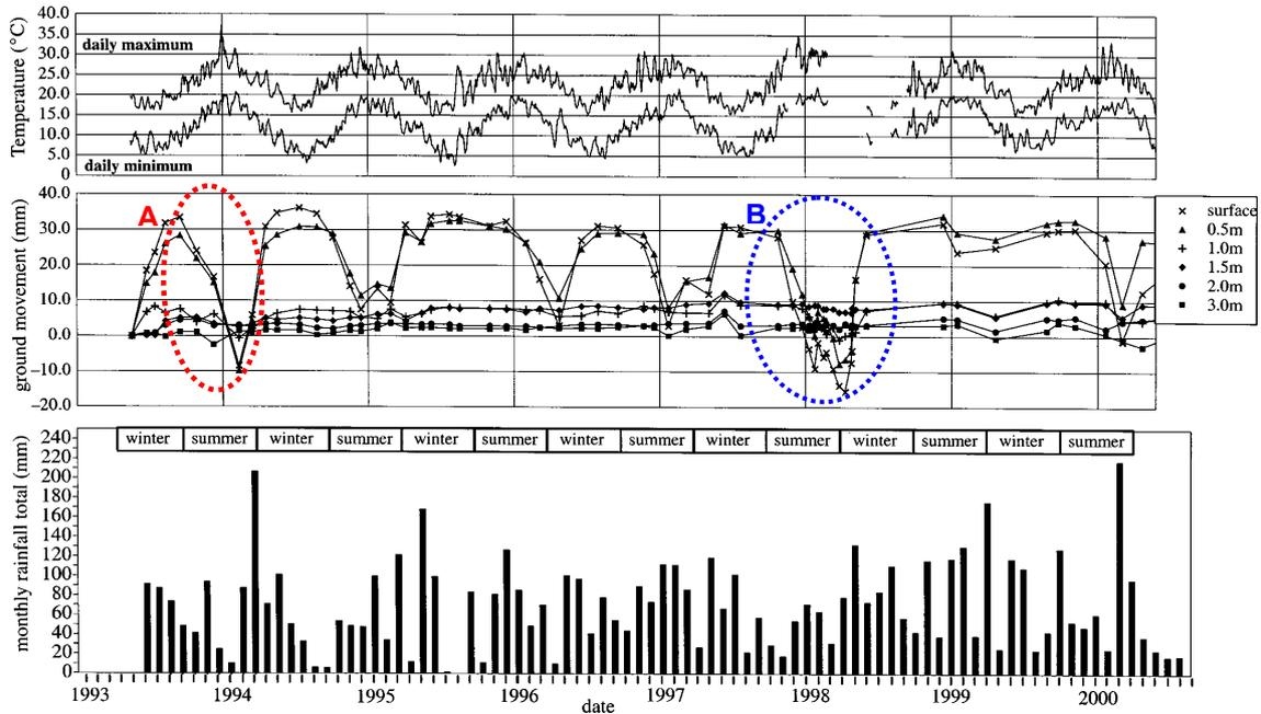
Figure 3. Data from Maryland field site, NSW, registered between 1993 and 2000. (a) Temperature (b) ground movements, (c) monthly rainfall (from Fityus et al, 2004)
