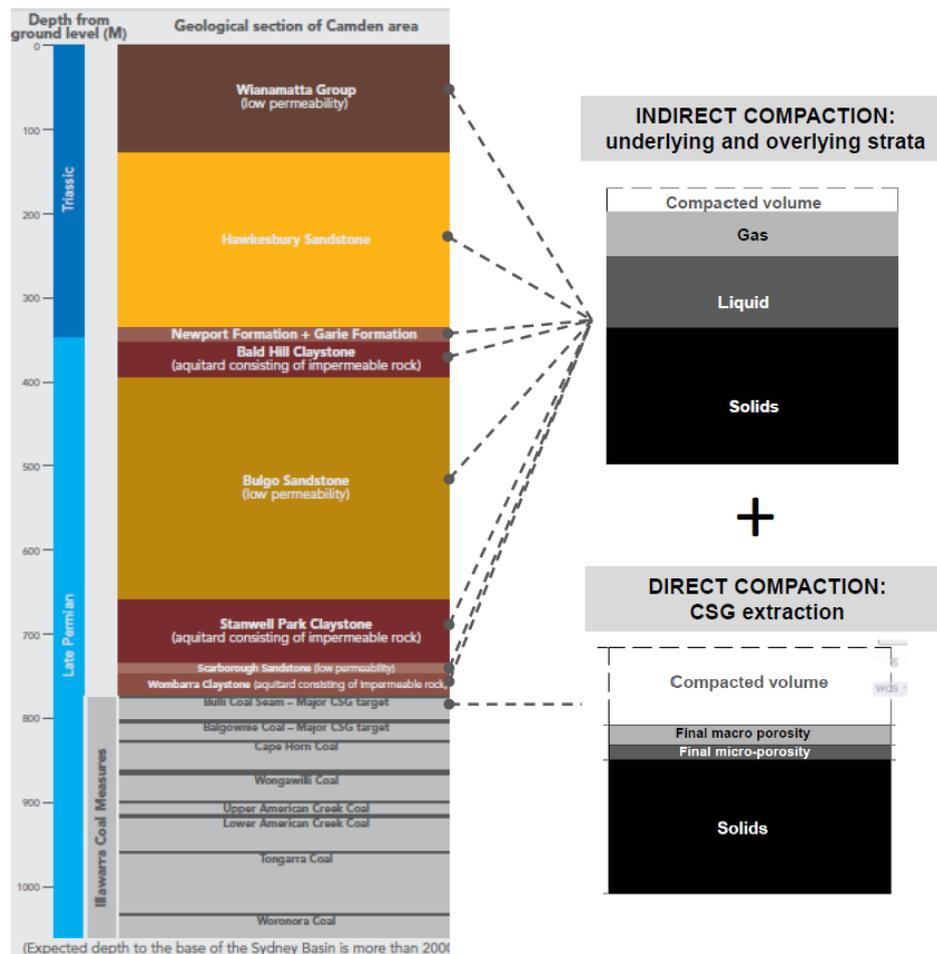
Figure 21. Geological profile at Camden Gas Project ([www.nsw.gov.au](http://www.nsw.gov.au)). Compaction process
