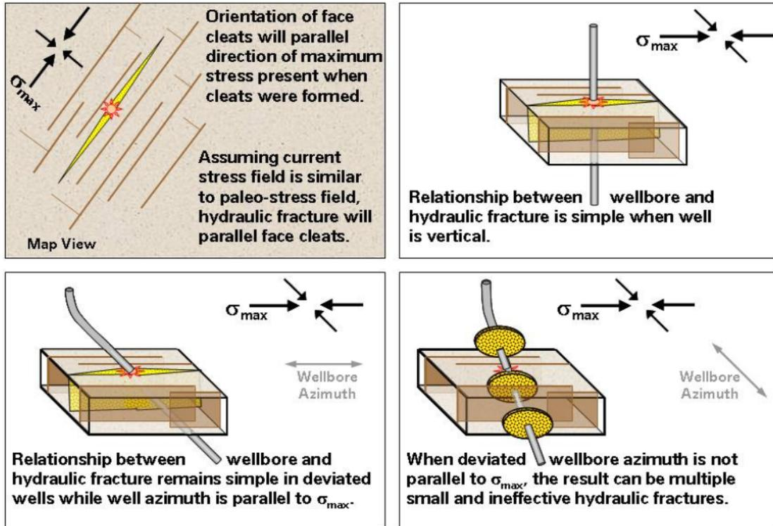
Figure 18. Relationship between the drilling procedure and the characteristics of the coal seam (from Loftin, 2009)
