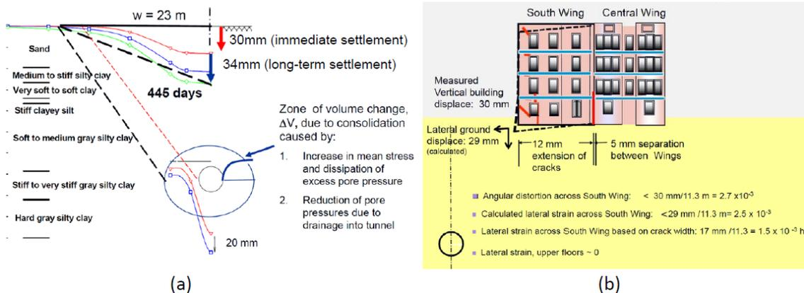
Figure 7. Consequences of tunnelling on buildings in Evanston. (a) Settlement trough. (b) Damage on a neighbour building (Cording et al, 2008).
