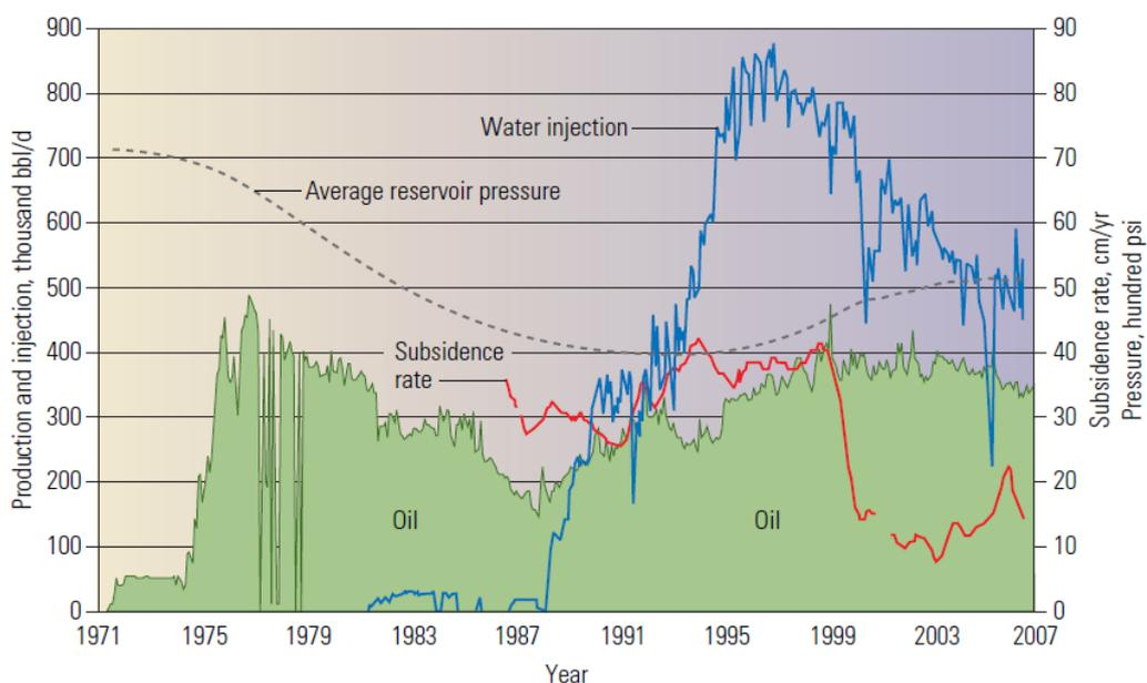
Figure 13. Variation of the reservoir pressure, subsidence rate and water-injected pressure at Ekofisk field-North Sea (from Doornhof et al, 2006)
