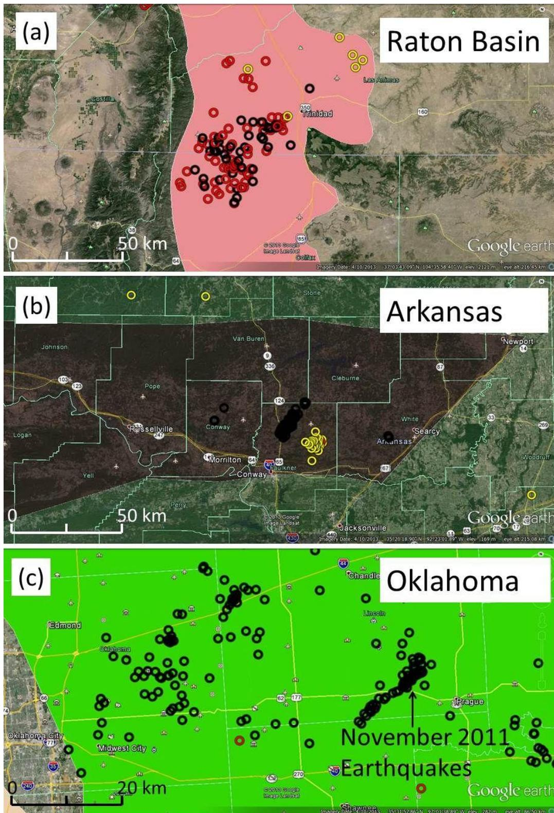
**Figure A4.4:** Distribution of earthquakes in three zones that experienced increased seismicity between 2001 and 2013. Bright red circles show earthquakes between 1973 and 2013. Very dark red circles are for earthquakes from 2001 to 2008. Black circles are for earthquakes between 2009 and 2013. (a) Raton Basin, (b) Arkoma Basin in Arkansas, (c) Cherokee Platform in Oklahoma.
