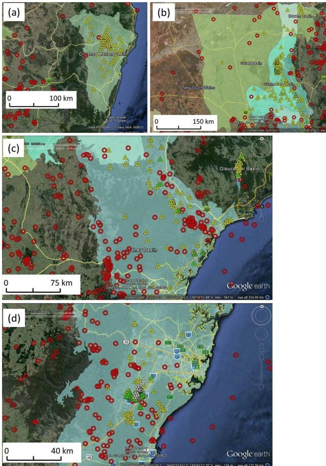
**Figure A5.3:** CSG wells and earthquakes in (a) Clarence Moreton Basin, (b) Southern Surat and Bowen basins and the northern Gunnedah Basins, (c) Southern Gunnedah and northern Sydney Basins and Gloucester Basin, and (d) Southern Sydney Basin. Wells are shown as triangles (Green – Hydrofractured; White – Production; Yellow – All other wells). Red circles are earthquakes; Diameter of circle reflects earthquake magnitude.
