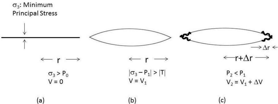
**Figure A2.3:** Three phases of crack development, based on Figure 1 of Secor (1968). (a) crack exists but is not filled with fluid and therefore has no finite volume; (b) crack has expanded under the influence of fluid pressure to the point where it is ready to fail at its tips; and (c) crack has failed at its at its tips and has become longer.
