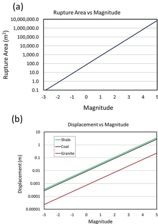
**Figure A3.2:** (a) Area of a circular rupture as a function of earthquake magnitude. (b) Displacement across a rupture as a function of earthquake magnitude for coal (black), shale (green) and granite (red) assuming a stress drop of 5 MPa and the shear moduli for the three rock types set out in Table A3.1.
