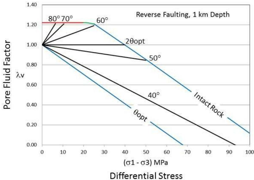
**Figure A2.4:** Failure mode diagrams for the reactivation of weak cohesionless faults as reverse faults compared to that for the creation of a new reverse fault in intact rock, for a number of values of misorientation of the existing faults from optimal to 80°. Red, green and blue curves are as for Figure A2.2
