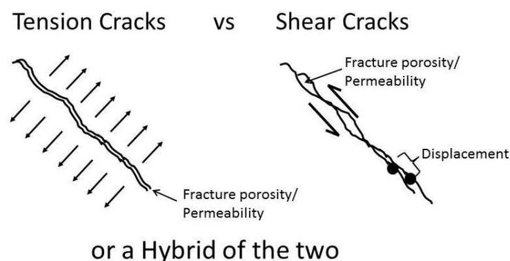
**Figure A2.1:** Modes of relative displacement of rocks on either side of a crack in rock.
