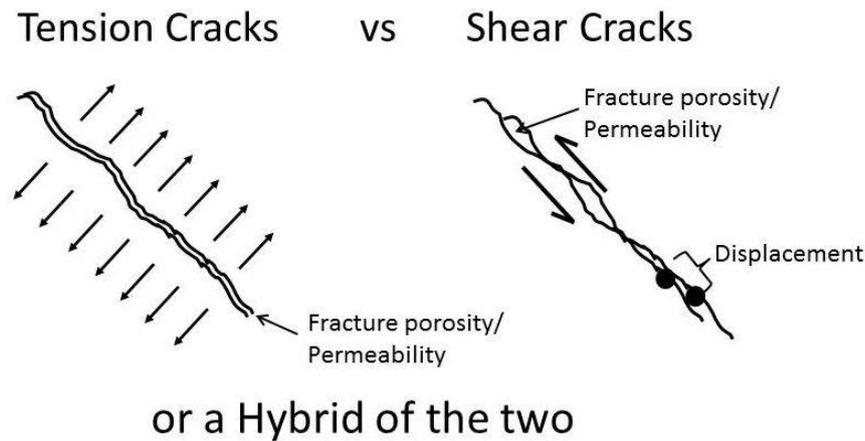
**Figure 3:** Diagrammatic representations of tension and shear cracks.
