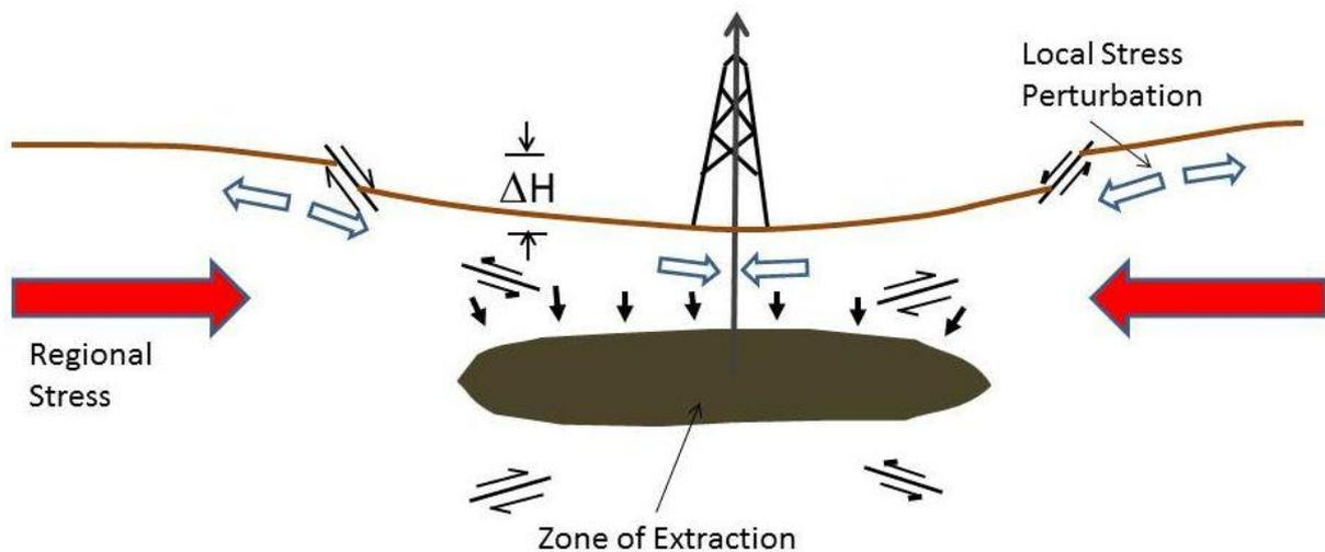
**Figure 6:** Perturbations in local stress (small open arrows) that are superimposed on the regional stress field (large red arrows) by the withdrawal of fluid from a reservoir, causing contraction of the reservoir and subsequent local surface subsidence. Thrust faults are induced under and above the reservoir and normal faults on the flanks. (after Segall, 1989, Figure 4).
