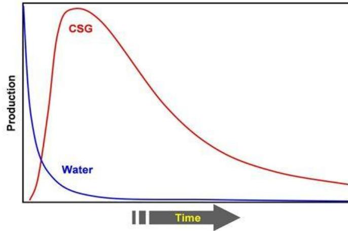
**Figure 7:** Withdrawal of water (blue curve) and production of gas (red curve) as a function of time for a coal seam gas well. The expected life of a coal seam gas well is 15 – 20 years. This figure:
