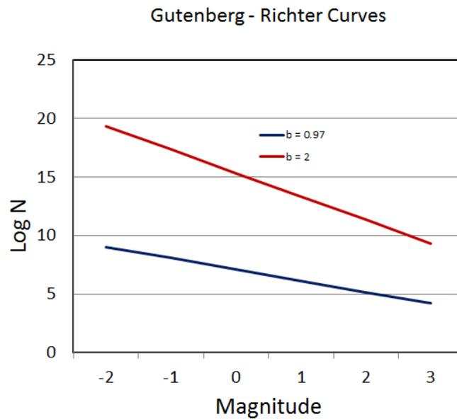
**Figure A3.3:** Graphical representation of the Gutenberg-Richter relation for earthquake size distribution. N is the number of earthquakes above a particular magnitude; b is the slope of the line: b=0.97 is typical of naturally occurring earthquakes; b = 2 is common in hydrofracture earthquakes.
