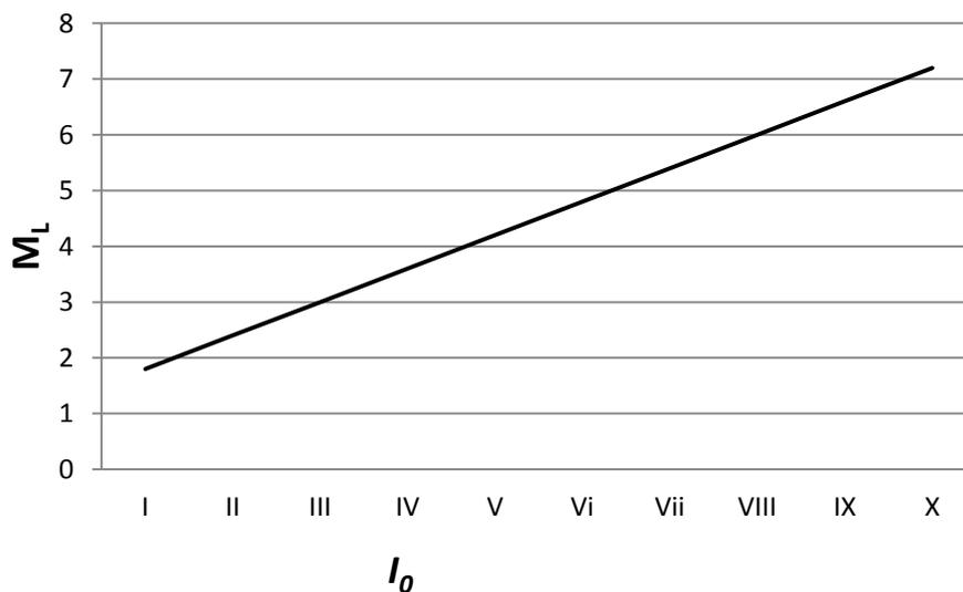
**Figure A3.1:** Richter magnitude vs intensity at the epicentre (for shallow earthquakes; ie, effectively near the hypocentre) for Australian earthquakes. Based on the relation in Equation 3, from Greenhalgh et al. (1988).
