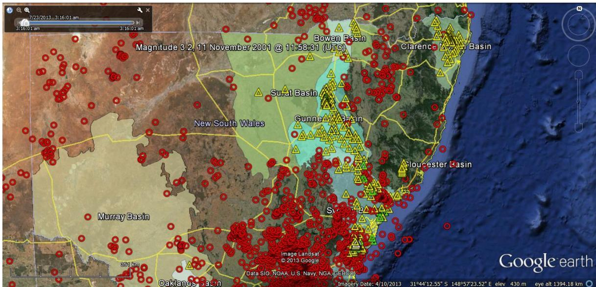
**Figure A5.2:** Locations of 556 CSG wells in New South Wales (Triangles: Green – Hydrofractured; White – Production; Yellow – all other wells). The locations of earthquakes in the national earthquake database maintained by Geoscience Australia are shown as red circles.
