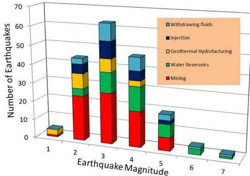
**Figure 5:** Histogram of earthquakes reported by Davies et al. (2013) as likely to have been induced, grouped according to human activities that would have caused a change in the stress regime, the fluid pressure regime, or both. The horizontal axis shows the magnitudes of the earthquakes in the Davies et al. (2013) catalogue; the vertical axis shows the number of earthquakes of each magnitude colour coded by category.
