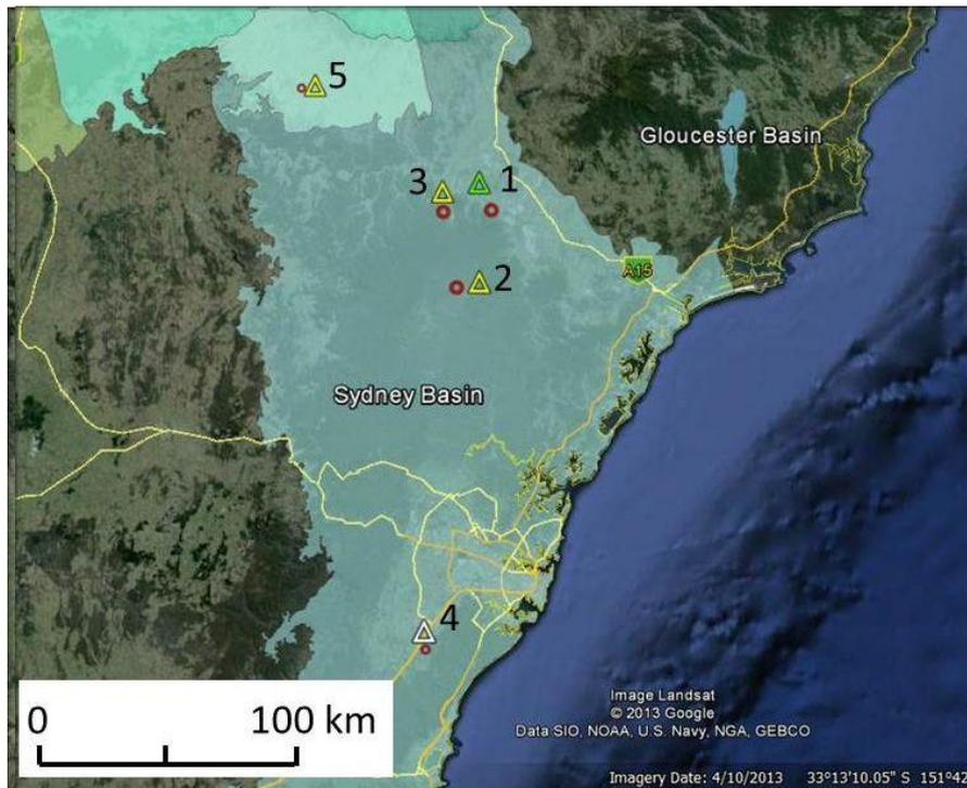
**Figure A5.4:** Five CSG wells (triangles) near which earthquakes (red circles) occurred during or shortly after the wells were drilled. Numbers beside the triangles refer to the well-earthquake pairs in Table A5.2 (above). Green triangles – hydrofractured; White – production; Yellow – all other wells.
