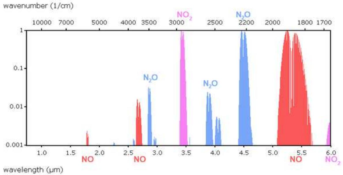
Figure 5: Absorption spectra of nitrous oxides (taken from <http://nanoplus.com/en/applications/applications-by-gas/nitrogen-oxides-detection-nox/>)
