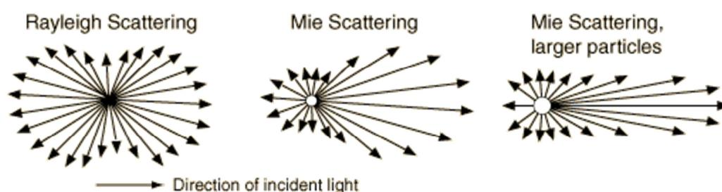
Figure 3: Directional patterns of Mie scattering and Rayleigh scattering (wavelength small compared to particle size)
