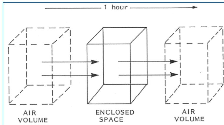
**Figure 2-1: Schematic representation of 1 ACH (Charlesworth, 1988)**
