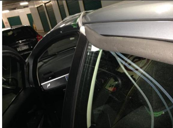
Figure C-7: Fiat Front Passenger Tube Setup (back view)
