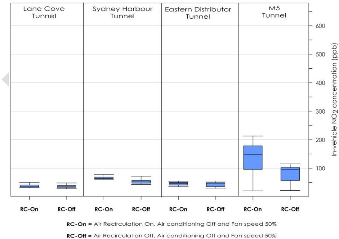
Figure E-5: In-Vehicle NO<sub>2</sub> concentration 2002 Audi A3 – Counter Direction
