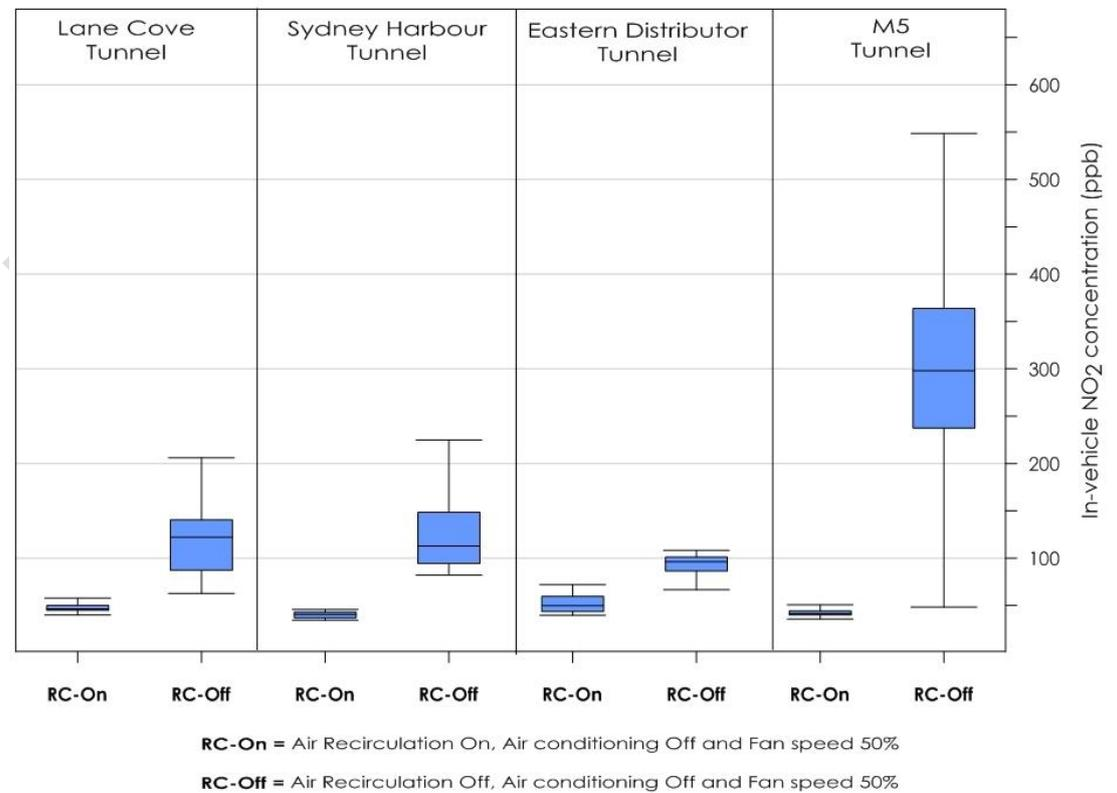
Figure E-3: In-Vehicle NO<sub>2</sub> concentration 2001 Subaru Outback – Counter Direction
