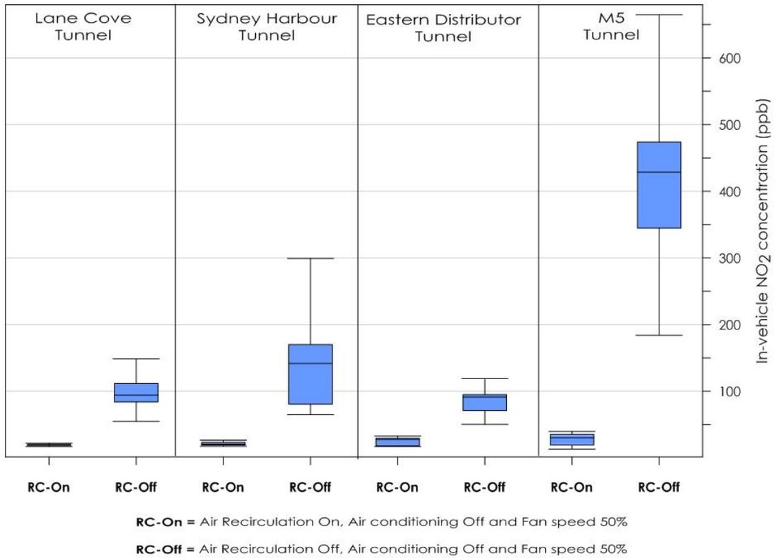
Figure E-4: In-Vehicle NO<sub>2</sub> concentration 2011 Toyota Corolla – Counter Direction
