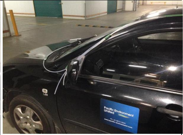
Figure C-14: Toyota Corolla passengers side tube setup
