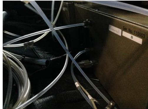
Figure C-11: Hyundai NO2 Cord Setup to NO2 Analyser
