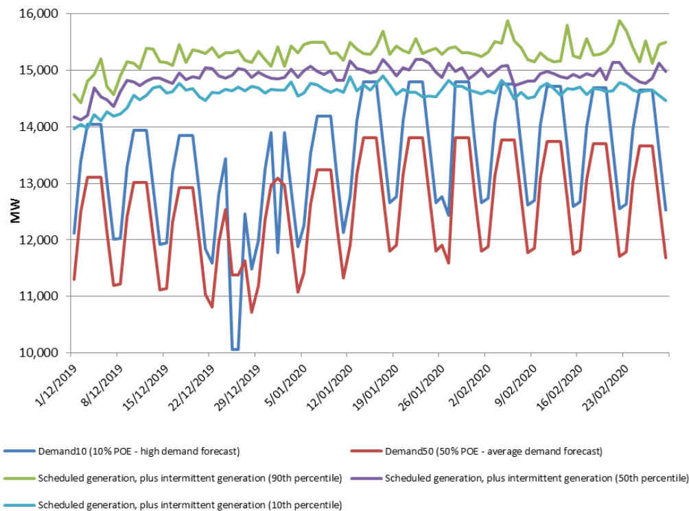
Figure 4: Comparison of NSW demand forecasts (10% and 50% POE) with scheduled and intermittent generation (at 10%, 50% and 90% intermittent)
