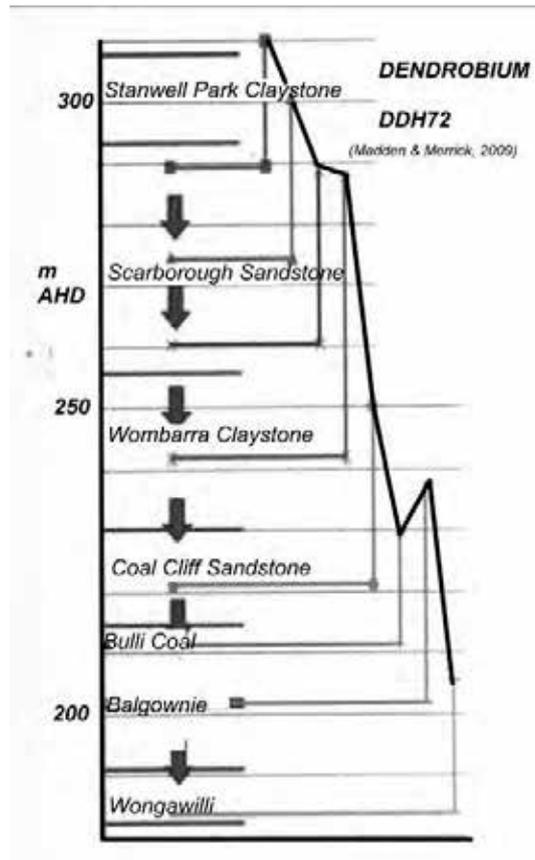
Figure 5 – Piezometric Profile, Southern Coalfields.
