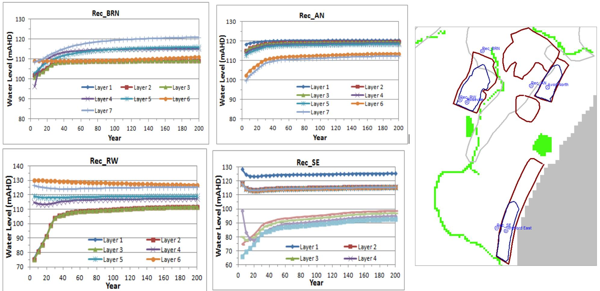
Figure A-55. Recovery Groundwater Hydrographs at Representative Sites
