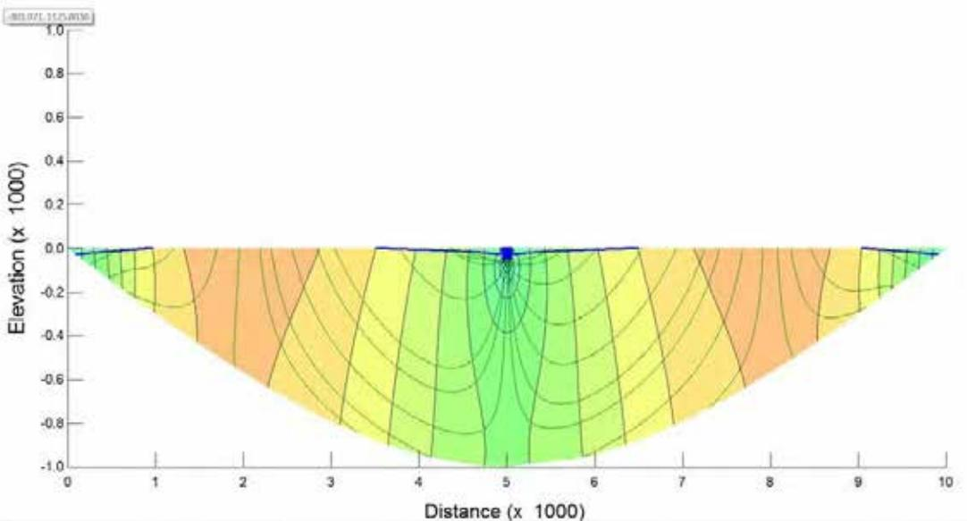
**Figure 13:** Flow lines and equipotentials if only fresh water in the basin.
