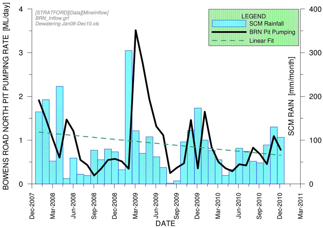
Figure A-21 Recorded Pumping Rates from the Bowens Road North Pit [ML/day]
