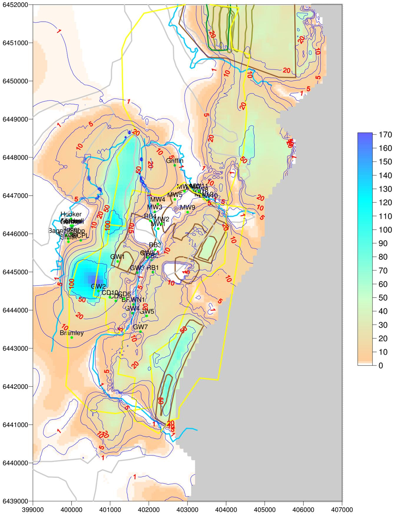
Figure A-58. Predicted Watertable Drawdown Contours Resulting from the Cumulative Effects of All Three Projects at 2024 [m]
