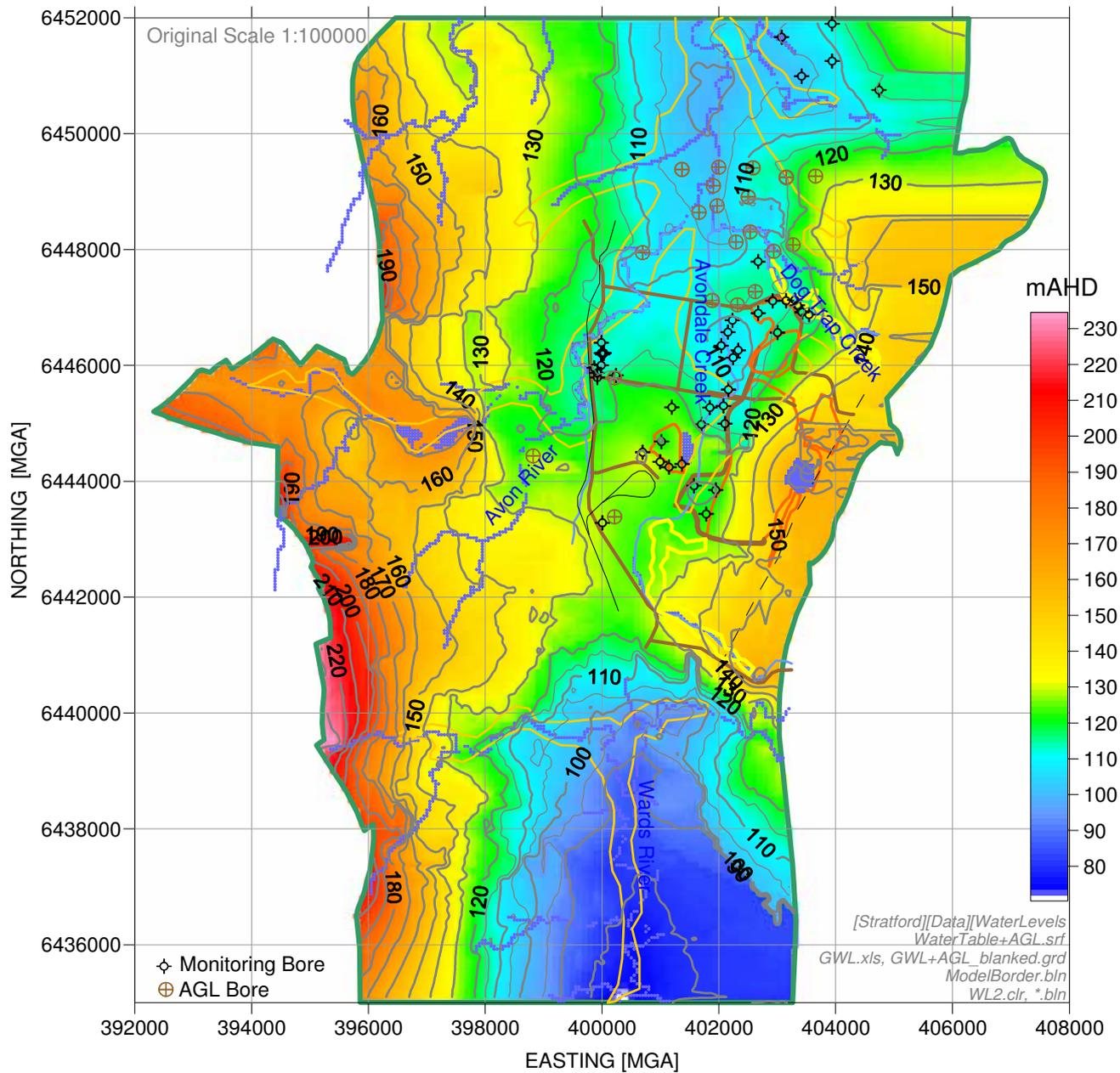
Figure A-16 Inferred Regional Shallow Groundwater Elevations [mAHD]
