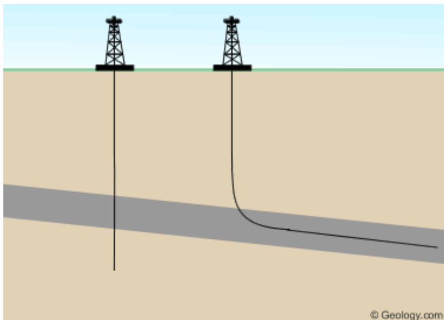
*Fig 8: The old and the new – a directionally drilled borehole*
