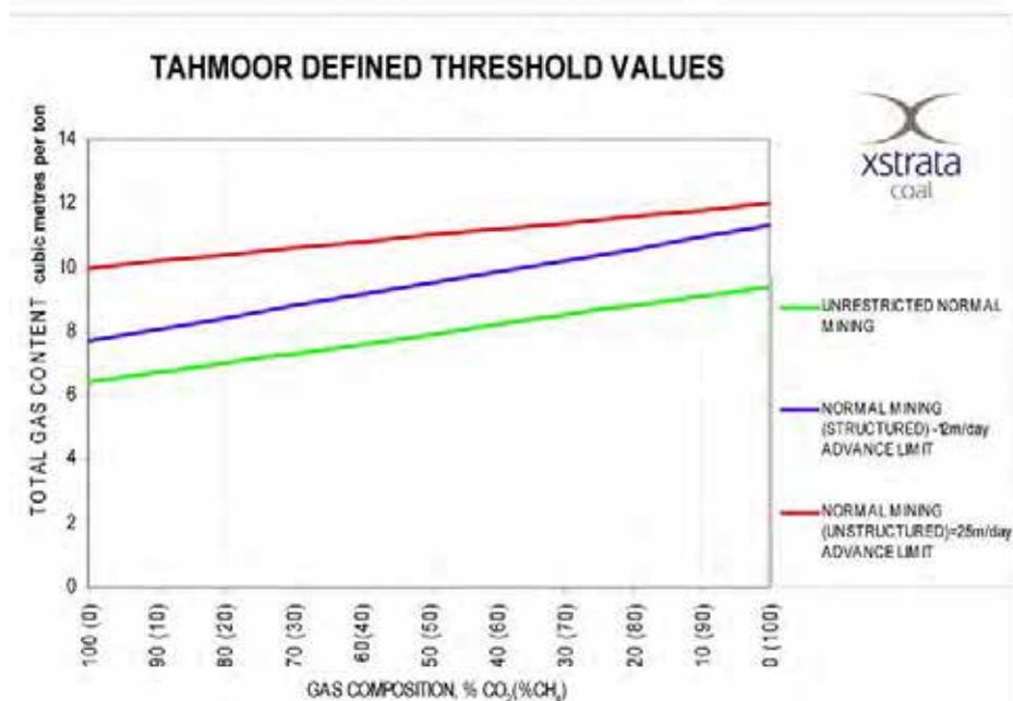
Fig 5: Drainage criteria for Tahmoor Colliery, NSW
