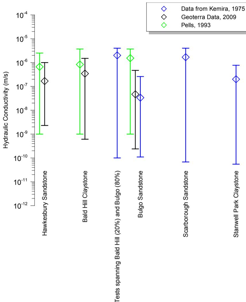
Fig 8 Hydraulic conductivity data for Triassic rocks of the Sydney Basin
