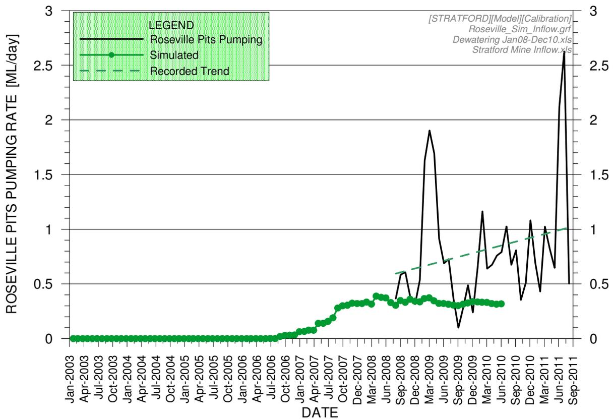
Figure A-40. Combined Roseville Pits Inflow Simulated during the Calibration Period
