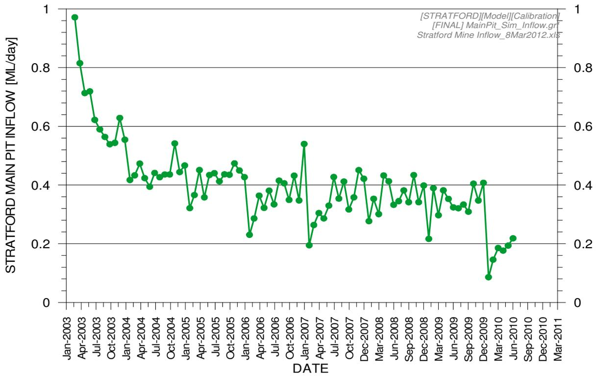
Figure A-41. Stratford Main Pit Inflow Simulated during the Calibration Period
