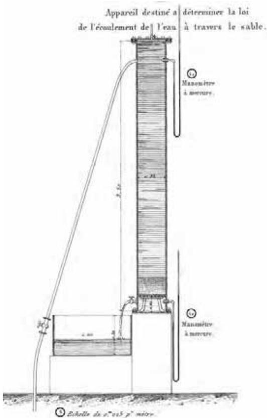
The test apparatus shown in Figure 11 is that used by Henry Darcy in 1855, from which were developed the widely used equations of groundwater flow.
