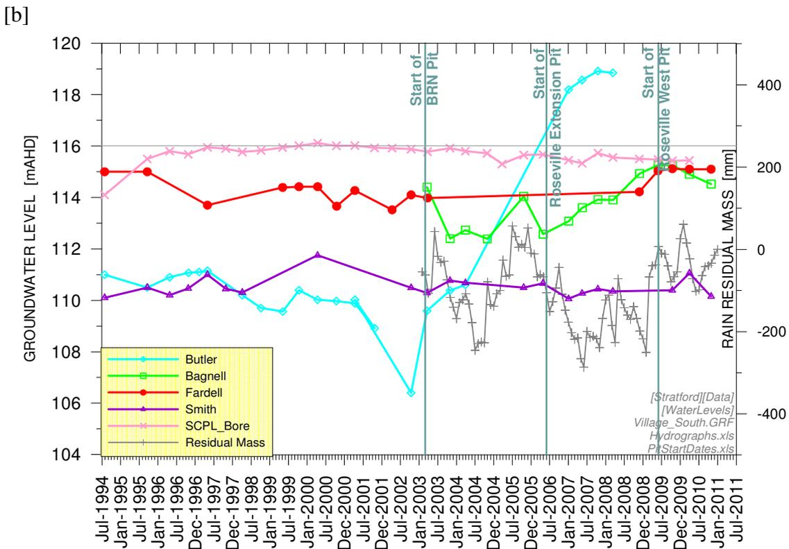
Figure A-20 Groundwater Hydrographs at Stratford Village: [a] north; [b] south
