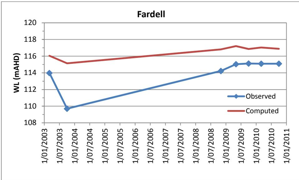
Figure A-46. Representative Simulated and Measured Hydrographs at Stratford Village [Bagnell and Fardell]
