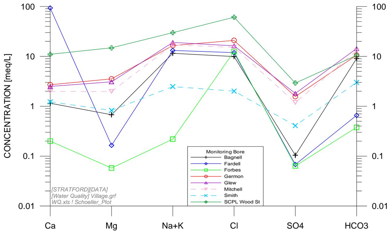
Figure AE-4. Schoeller diagram for major ions in interburden at Stratford Village
