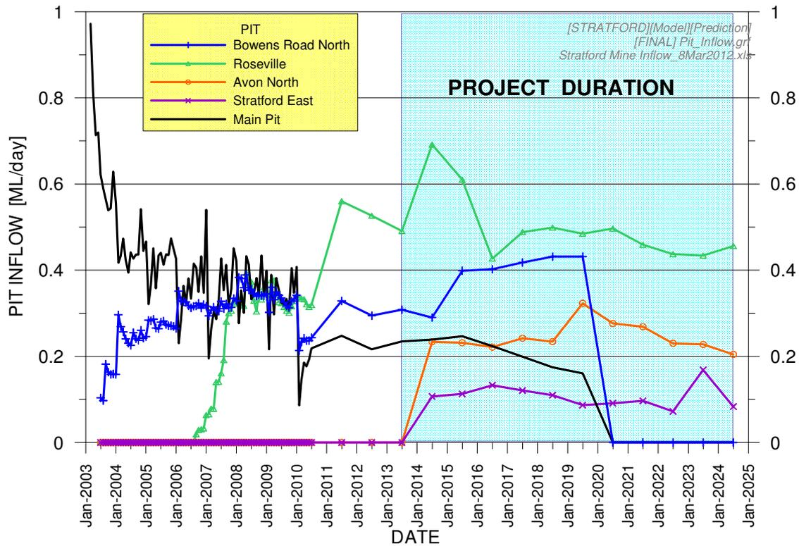
Figure A-47. Simulated Groundwater Inflow to Each Pit
