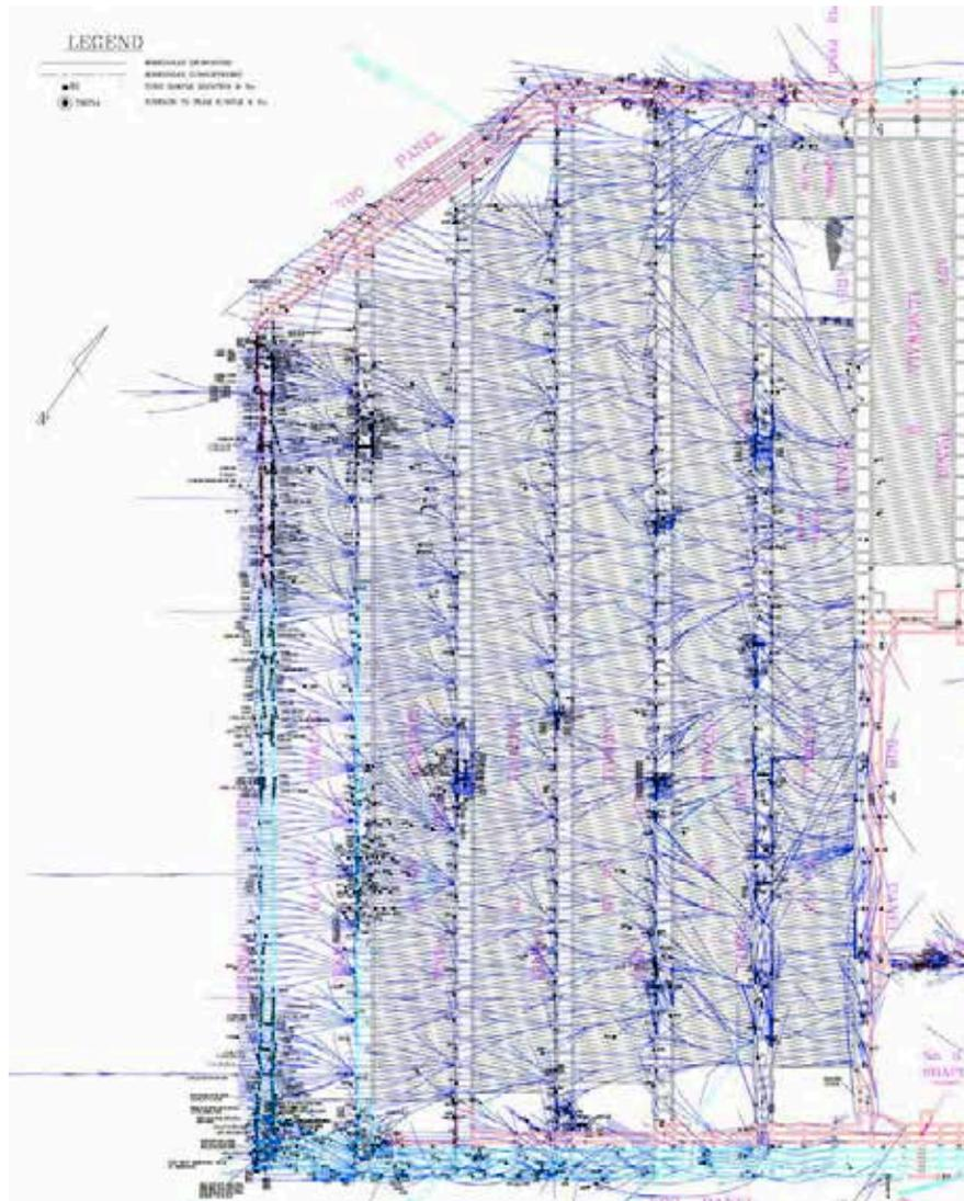
Fig 6: Example of in-seam gas drainage holes.
