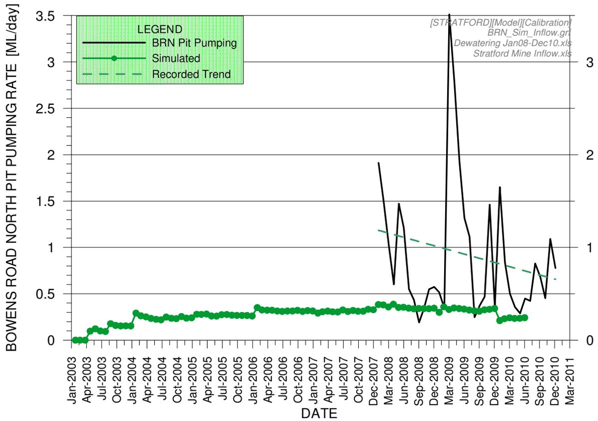
Figure A-39. BOWENS ROAD North Pit Inflow Simulated during the Calibration Period
