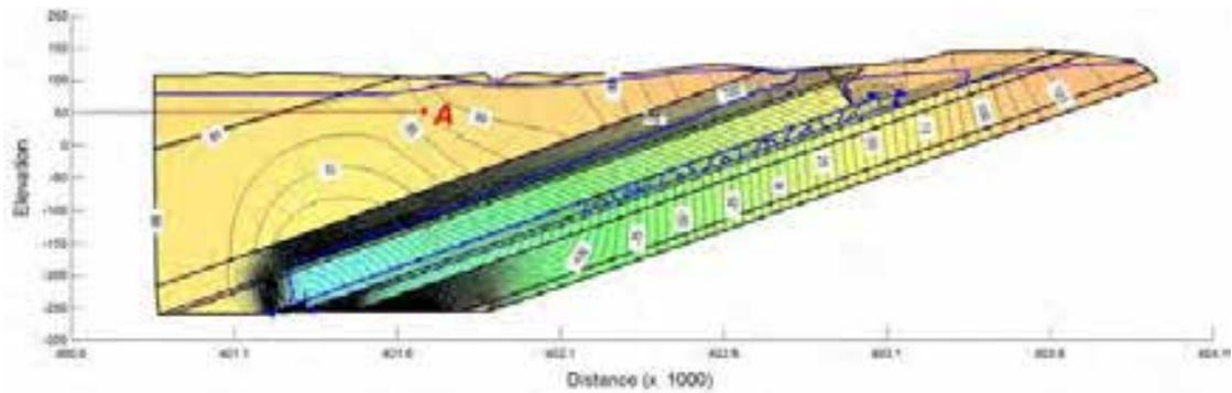
**Figure 16:** Equipotentials 2 years after CSG depressurisation in Deards Seam only.
