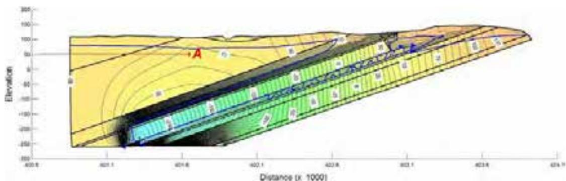
**Figure 17:** Equipotentials 20 years after CSG depressurisation in Deards Seam only.
