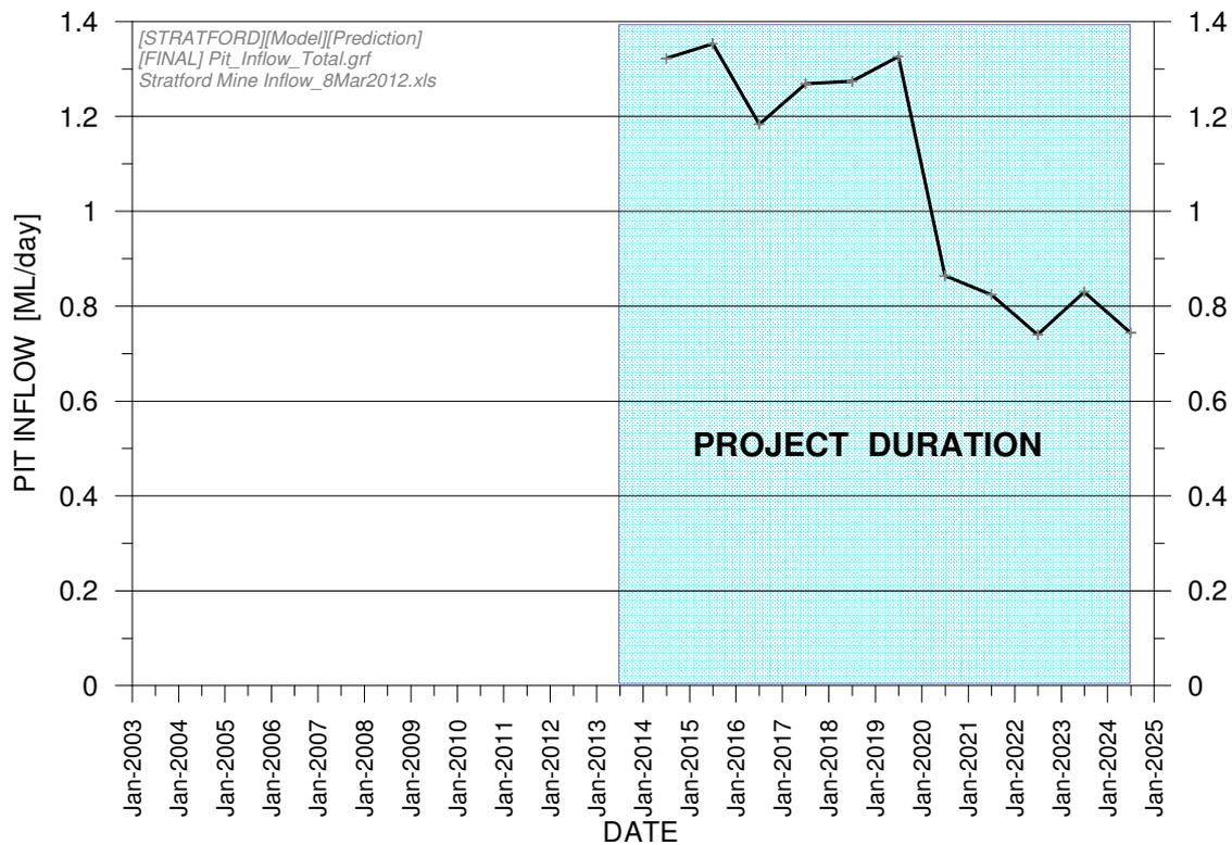
Figure A-48. Simulated Total Groundwater Inflow to Bowens Road North, Roseville, Avon North and Stratford East Pits during the Project
