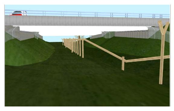
Fig 4. 3D Model of typical 15m plank bridges for koala connectivity
