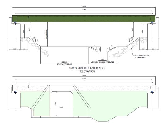
Fig 6: Comparison of culvert openings to plank bridges.
