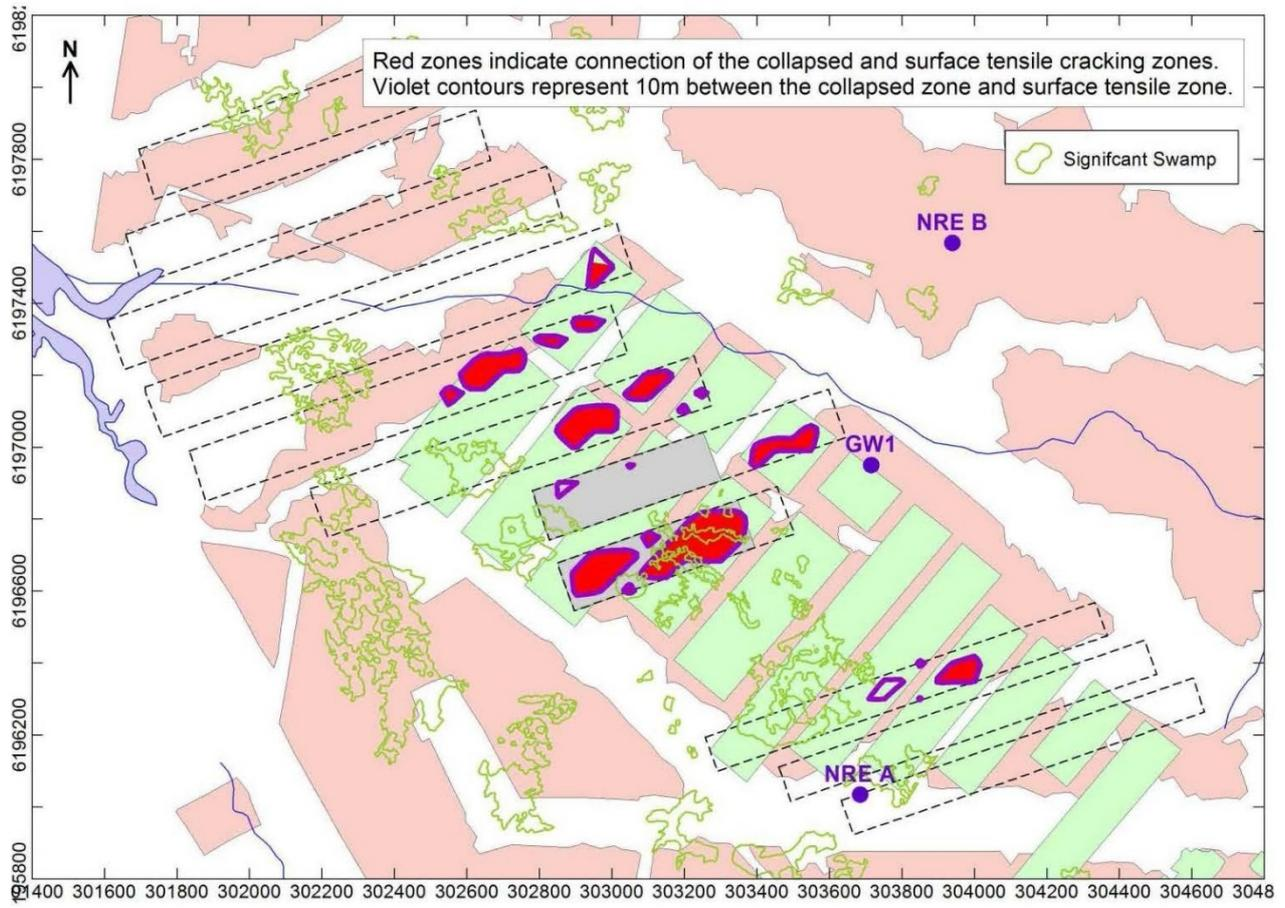
**Figure 57.** Tammetta’s depiction of areas where the drainage zone above triple seam extractions would reach the surface at the Russell Vale Colliery.
