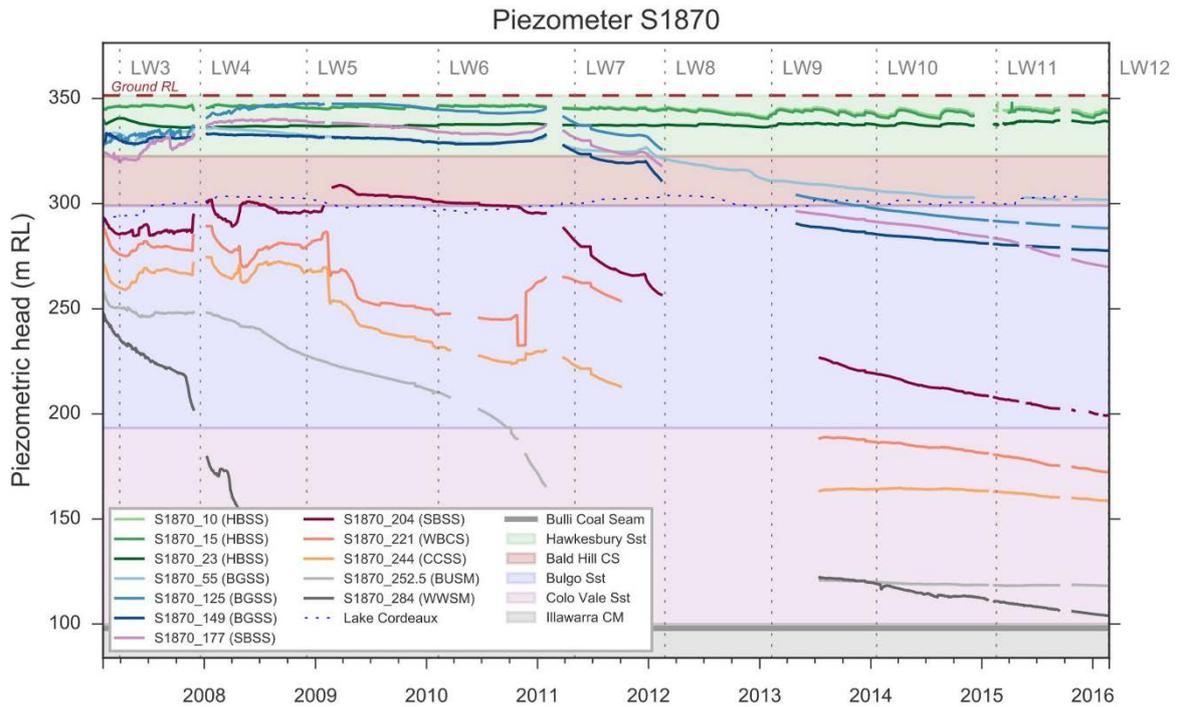
**Figure 35.** Hydrographs from piezometer bore DDH85/S1870
