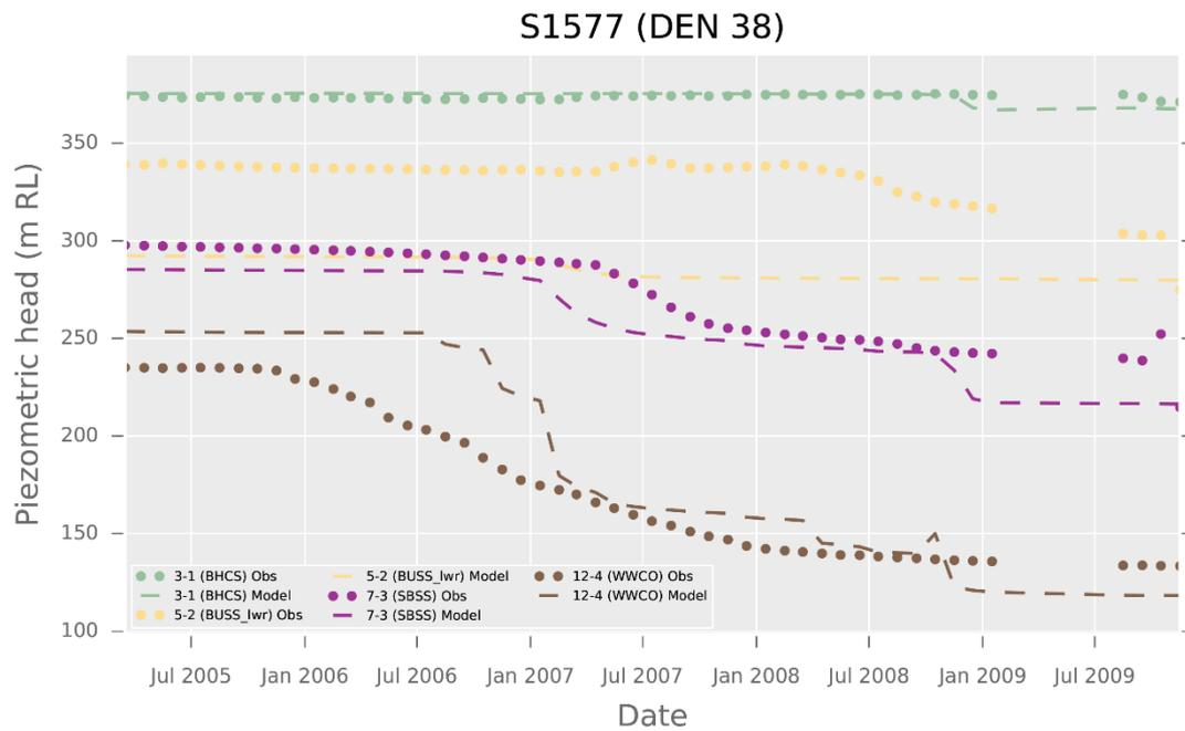
**Figure 30.** DDH38 piezometer hydrographs from the March 2016 HydroSimulations groundwater impact assessment[24] for Area 3B of the Dendrobium mine.
