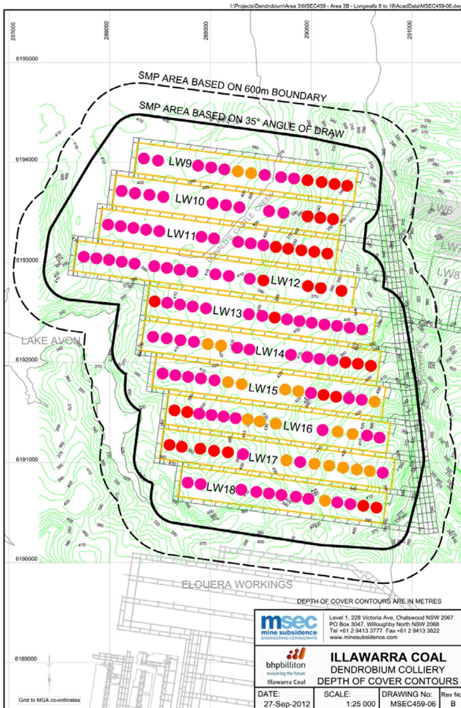
**Figure 20.** Depiction of the height of the drainage zone for 4.0m high extractions in Area 3B
