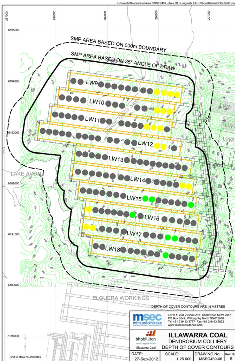
**Figure 18.** Depiction of the height of the drainage zone for 3.0m high extractions in Area 3B
