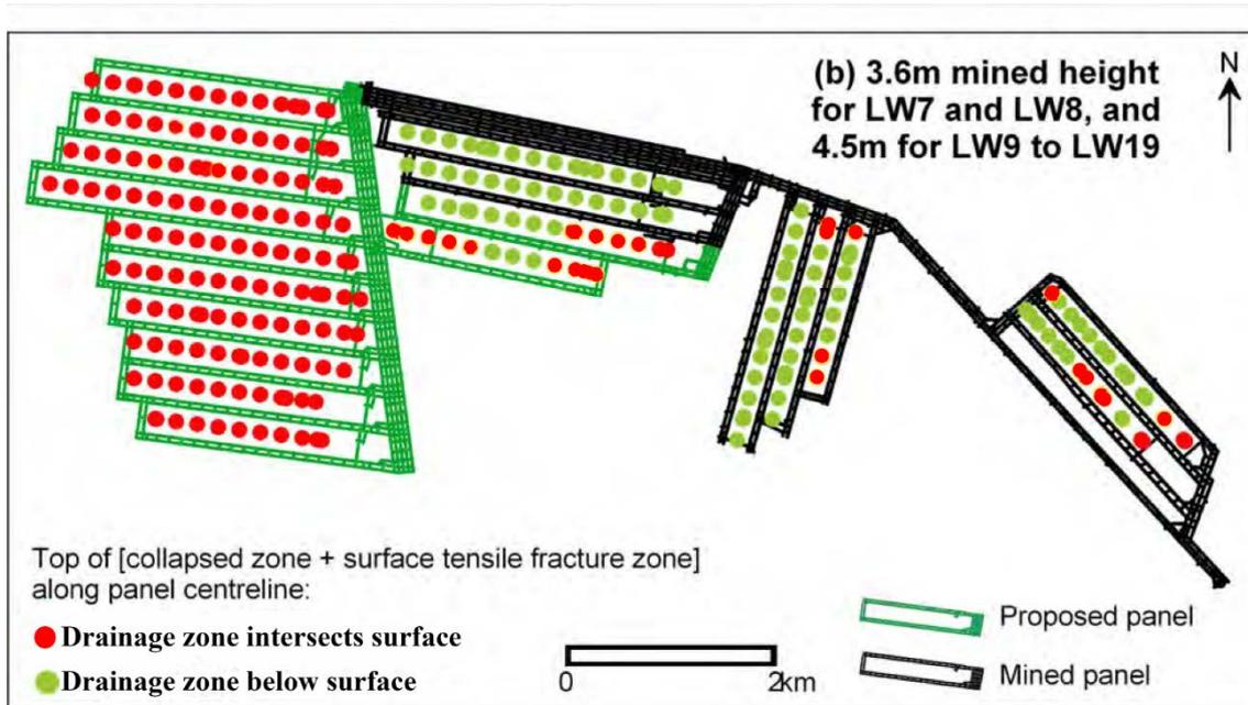
**Figure 23.** Tammetta depiction for Coffey Geotechnics of relationship of drainage zone height estimates with respect to the surface above the longwalls of Dendrobium Area 3B.
