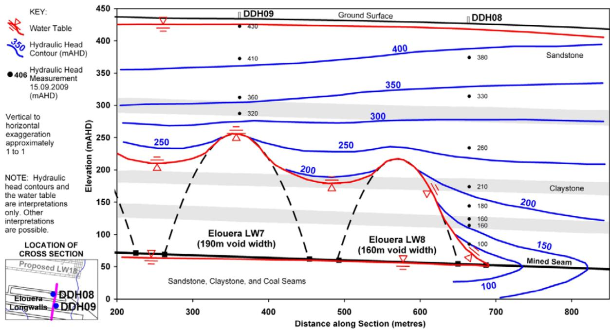
**Figure 15.** Hydraulic head measurements and Tammetta interpreted contours for Elouera LW 7
