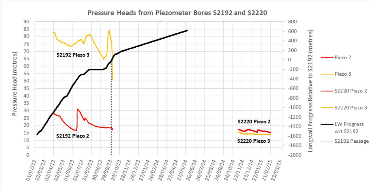
**Figure 45.** Pressure heads from S2192 and S2220 piezometers 2 and 3
