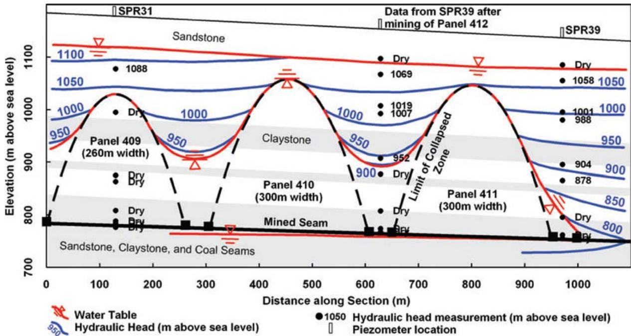
**Figure 13.** Hydraulic head measurements and Tammetta[16] interpreted contours for Springvale
