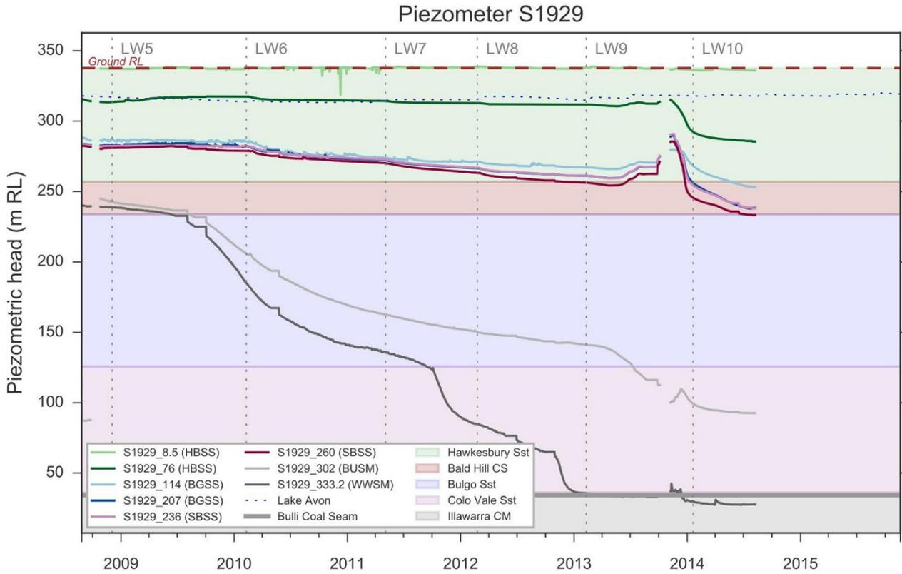
**Figure 46.** DDH111/S1929 hydrographs from the Longwall 11 end of panel report.[73]
