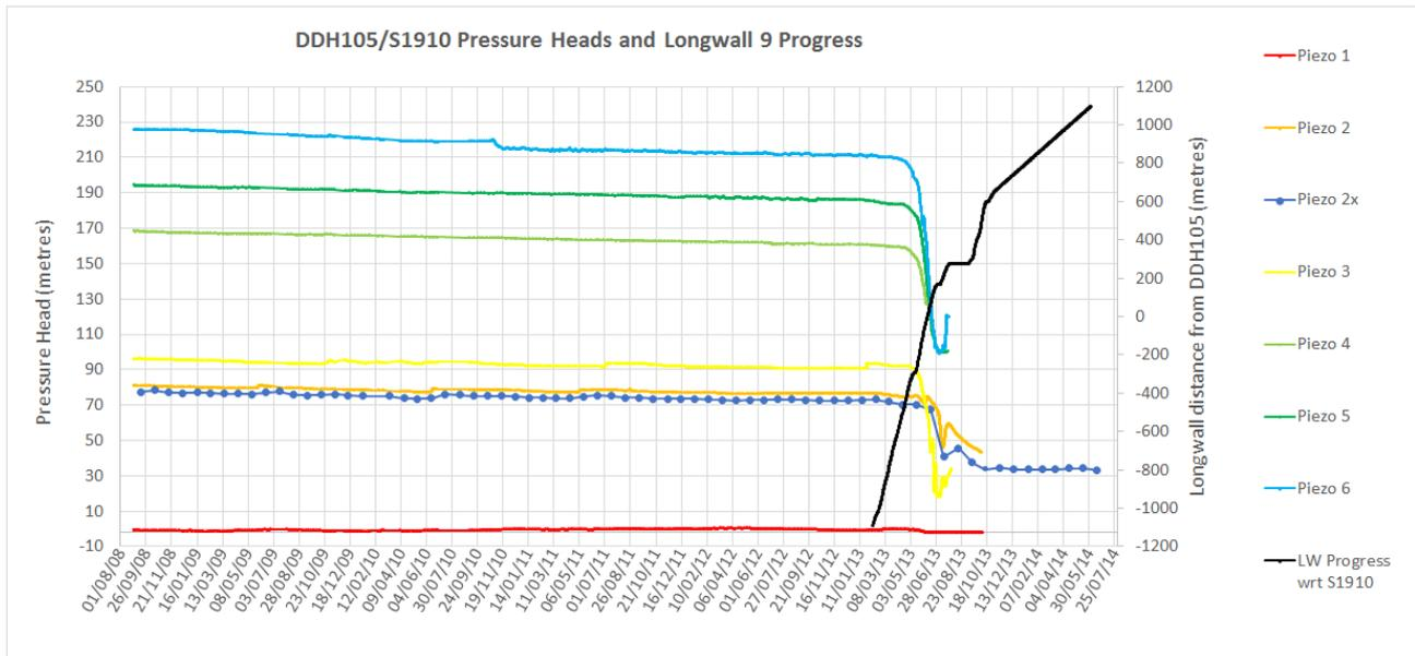
**Figure 37.** Pressure heads for Piezometers 2 to 6 in off-panel bore DDH105/1910 near Longwall 9 of Dendrobium Area 3B.
