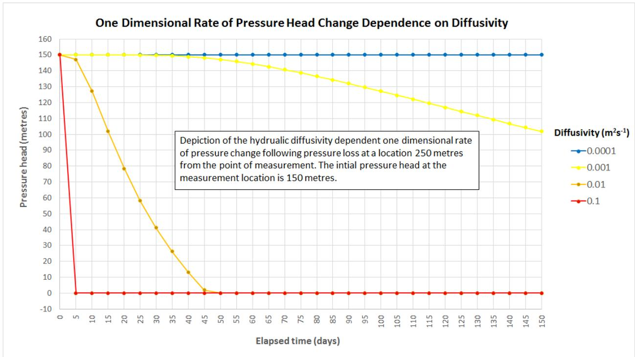
**Figure 1.** Pressure change with time dependence on hydraulic diffusivity
