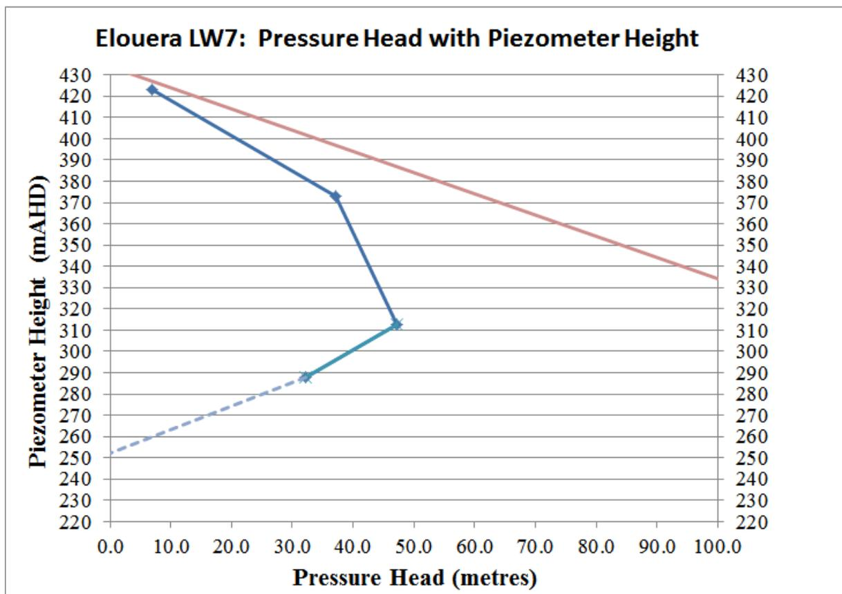
**Figure 16.** Height of the drainage zone obtained from Elouera LW7 piezometer data
