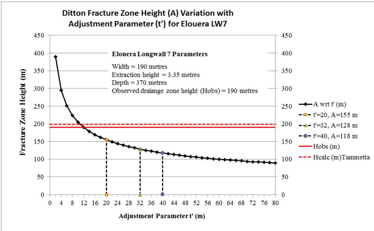
**Figure 8.** Variation of Ditton fracture zone height estimate with adjustment parameter  $t'$
