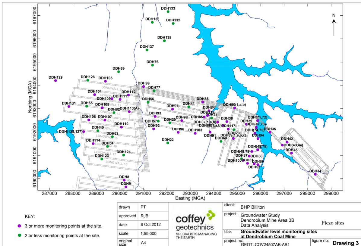
**Figure 28.** Coffey map showing the location of the piezometer bores used for model calibration by Tammetta.
