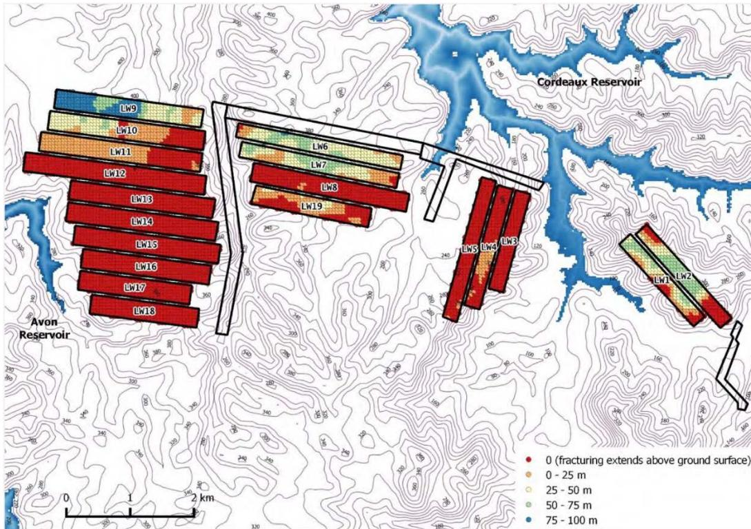
**Figure 22.** HydroSimulations 2015 depiction of Tammetta equation drainage zone height estimates for Area 3B of the Dendrobium mine.
