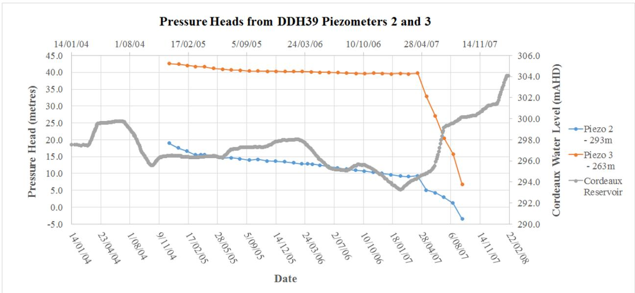
**Figure 26.** Pressure heads recorded by Piezometers 2 and 3 in bore DDH39 over Longwall 3 in Area 2 of the Dendrobium mine.
