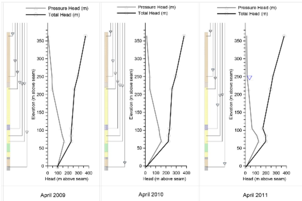
**Figure 34.** DDH97/S1889 piezometer pressure head profiles with respect to elevation.
