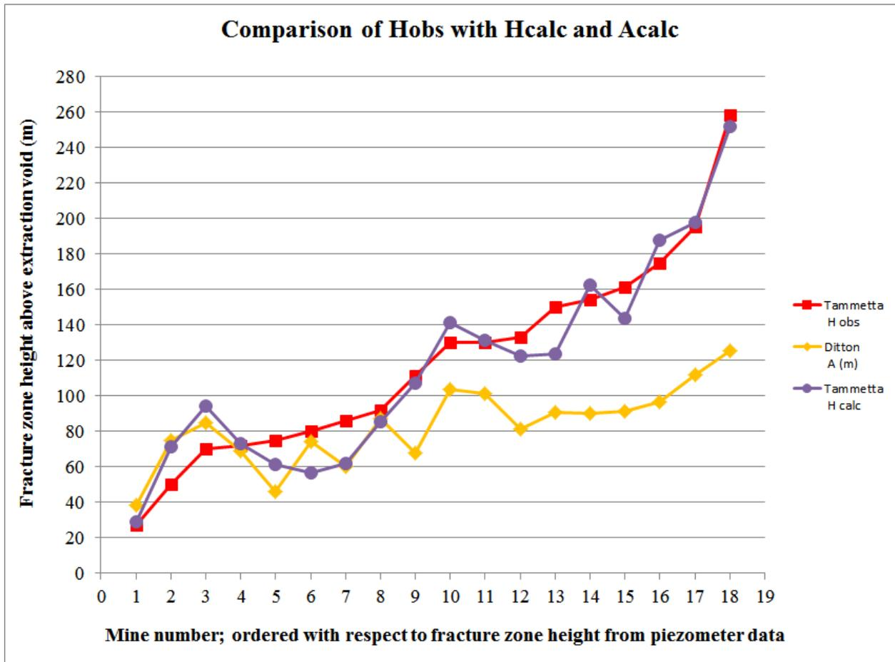
**Figure 5.** Comparison of Hcalc and Acalc with respect to Tammetta’s database
