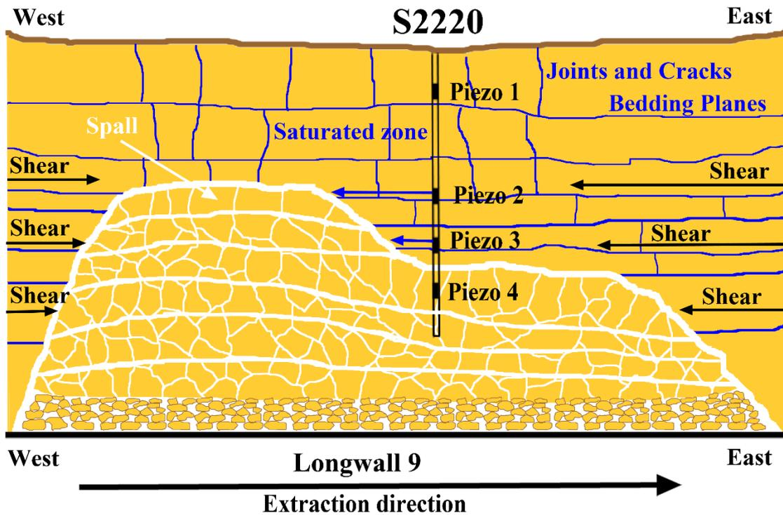
**Figure 53.** A west to east depiction of the drainage zone over Longwall 9 in Area 3B of the Dendrobium mine.
