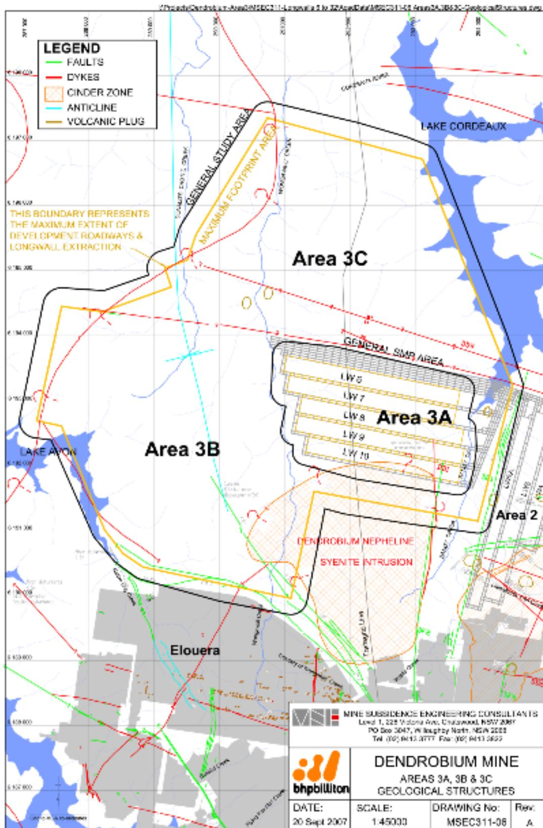
**Figure 9.** Geological structures in the vicinity of the Elouera domain and Dendrobium Area 3B
