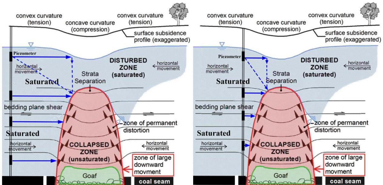
(a) Off-panel piezometer bore
