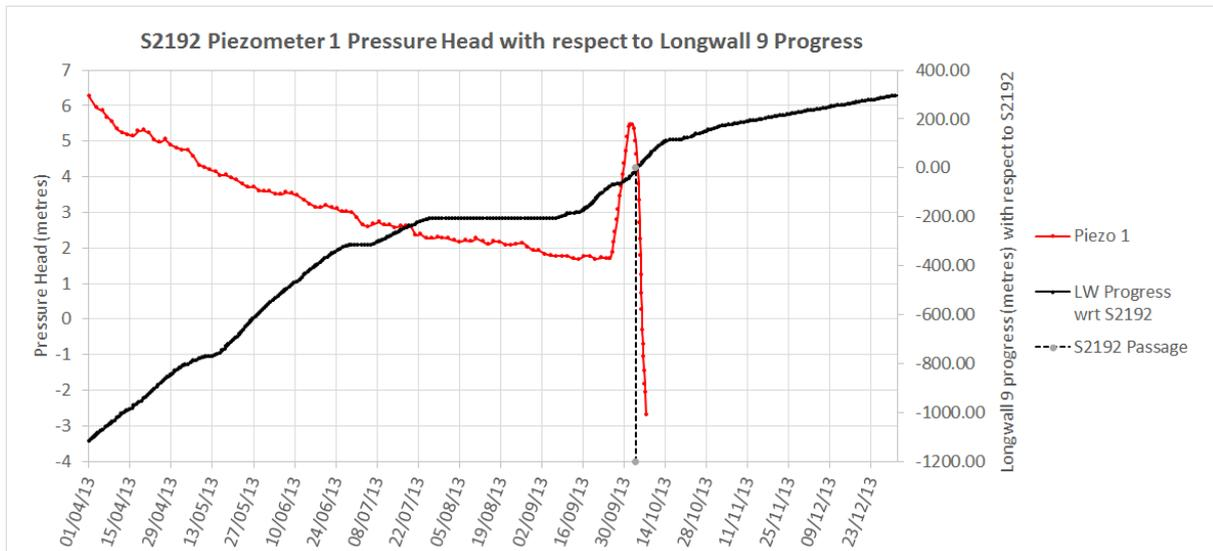
**Figure 44.** Pressure heads from S2192 piezometers 1 and Longwall 9 progress
