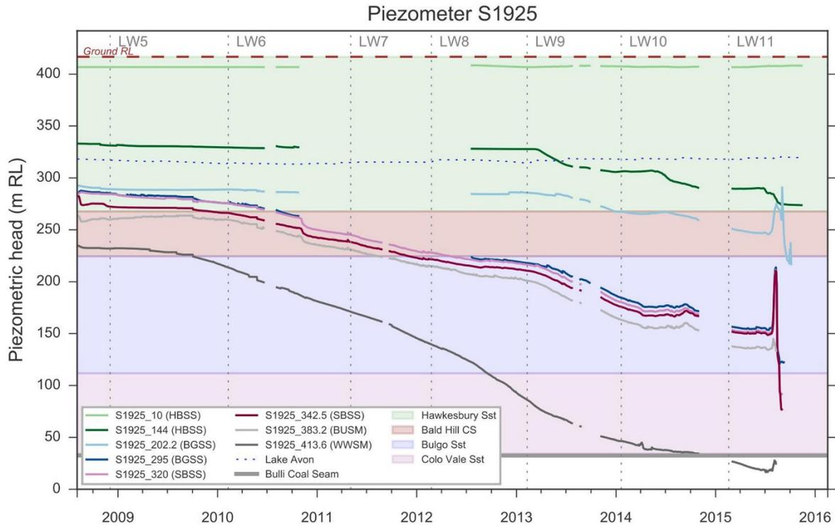
**Figure 48.** DDH108/S1925 hydrographs from the Dendrobium Longwall 11 end of panel report
