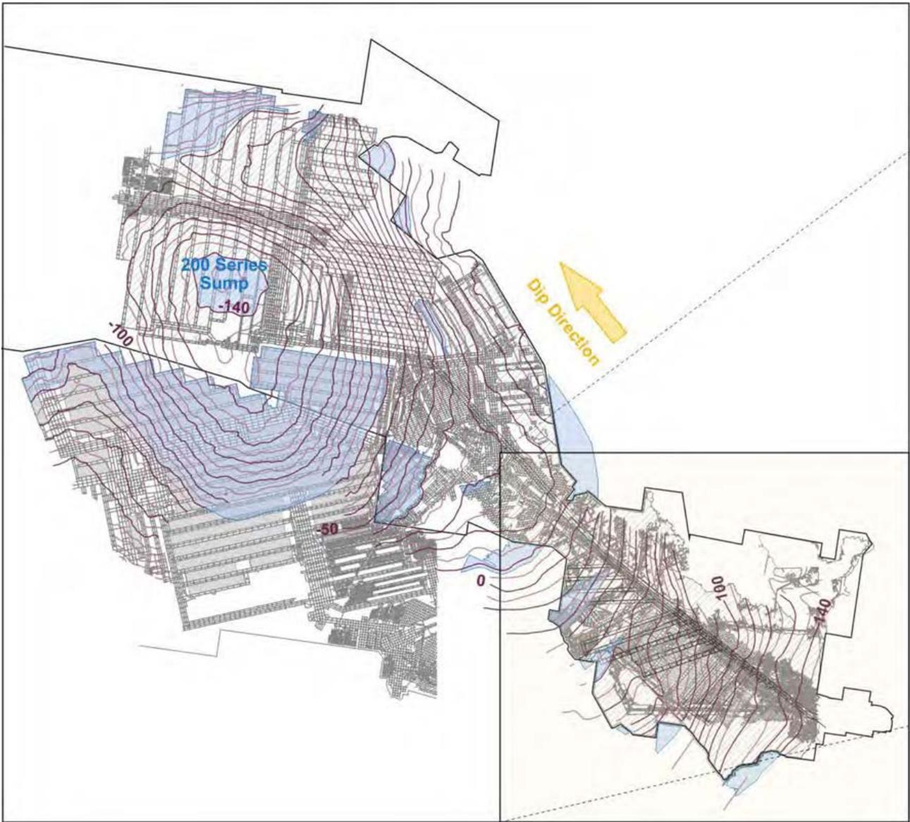
**Figure 60.** SCT schematic showing the flooded areas of the Russell Vale, Cordeaux-Corrimal and Bulli mines.
