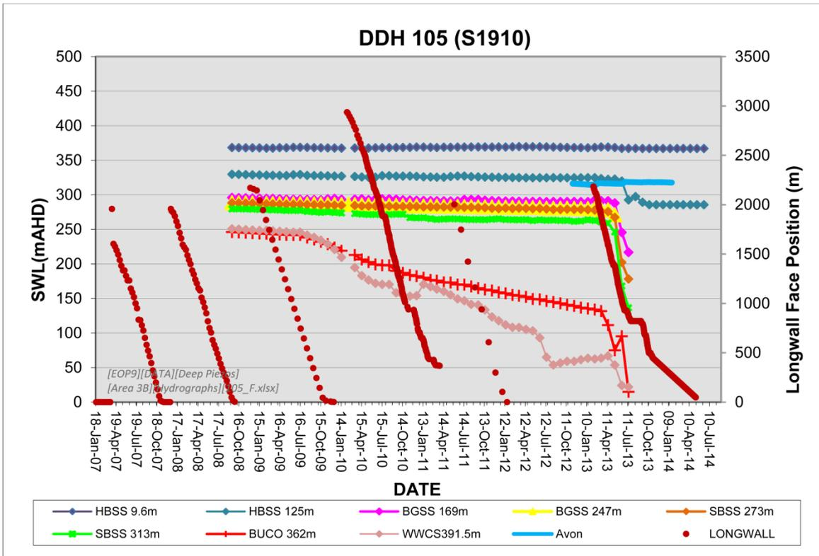
Figure 2.6 Groundwater hydrographs for Bore S1910 in Area 3B (LW9)
