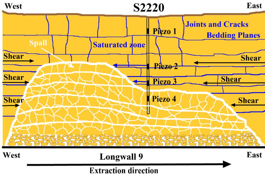
**Above figure:** qualitative depiction of a lengthwise drainage zone profile for Longwall 9 in Area 3B of the Dendrobium mine that could account for data from post-extraction centreline bore S2220, pre-extraction centreline bore S2192 (approx. 18m south of S2220) and off-panel bores S1910, S1925 and S1929 (not shown) over Area 3B. See Sections 15 and 16 within.
