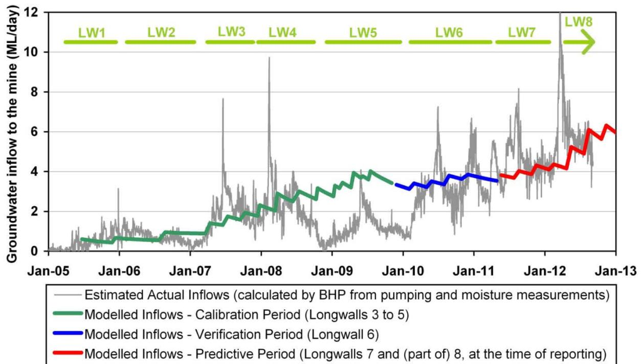
**Figure 19. Calibrated groundwater inflows to the Dendrobium mine.**
