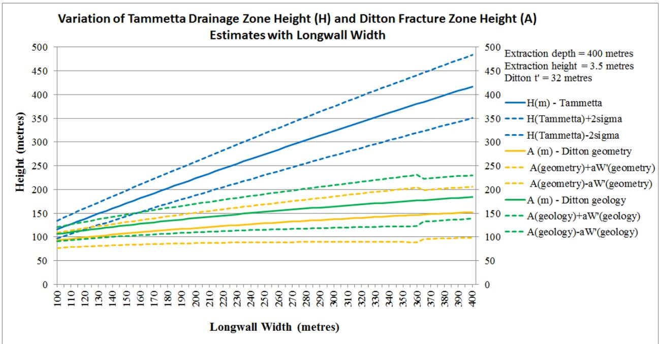
Figure 6. Tammetta and Ditton equation height estimate variation with longwall width.
