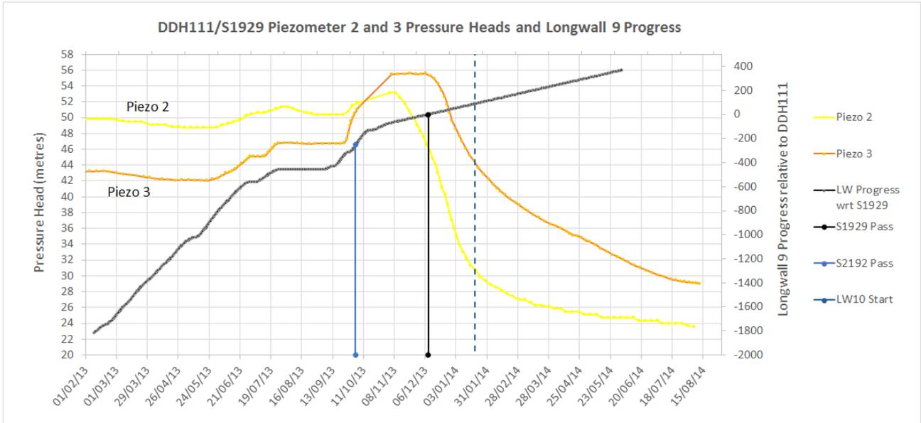
**Figure 47.** DDH111/S1929 Piezometer 2 and 3 pressure head profiles
