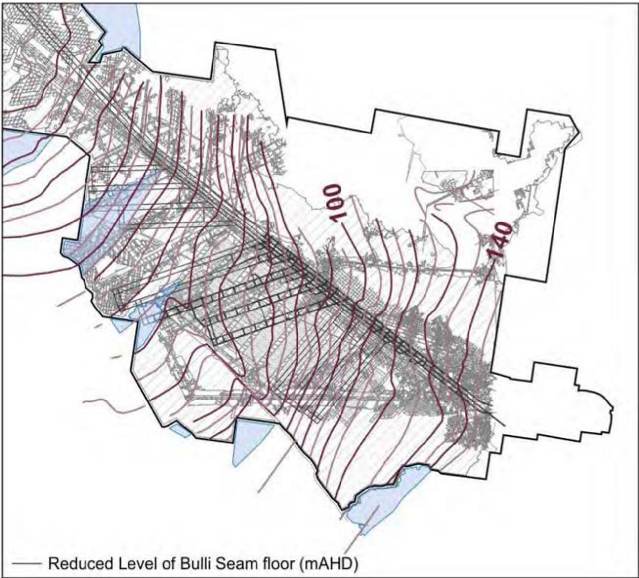
**Figure 61.** Expanded Fig. 60 inset showing water accumulation areas in the eastern domain of the Russell Vale Colliery.
