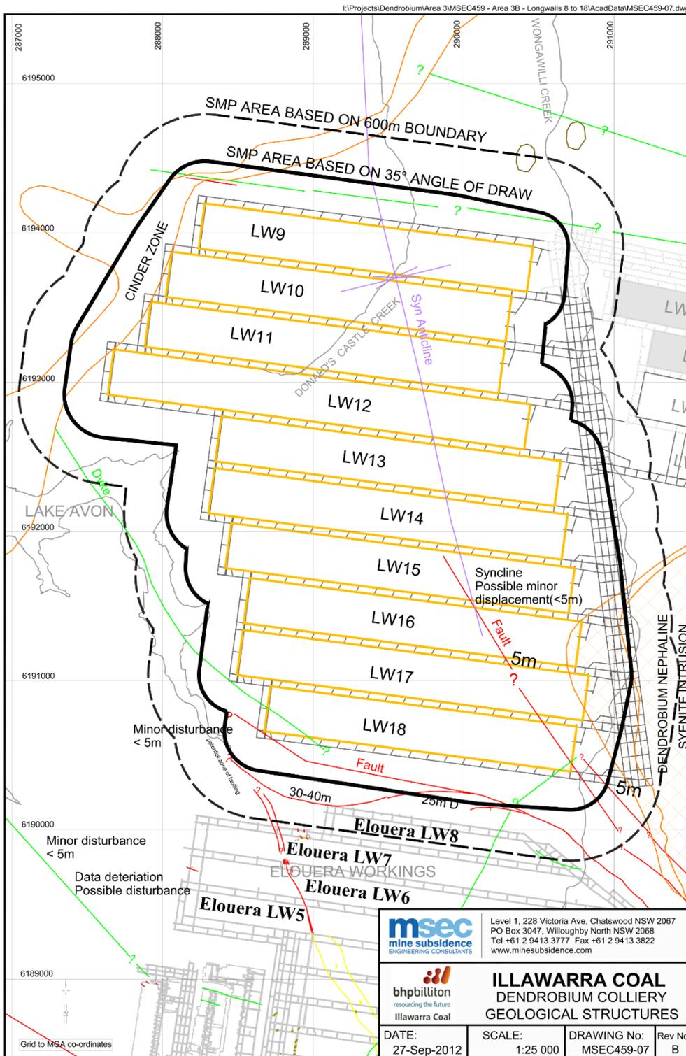
**Figure 10.** Proximity of Elouera Longwalls and geological structures over the Area 3B longwalls MSEC[61] depiction of geological structures over the Area 3B longwalls. An unusual nephaline syenite formation slightly intrudes in to the south eastern corner of Area 3B. There are no other noteworthy Area 3B deviations from the stratigraphy typical of the Woronora Plateau (see Fig. 11). Labels for the Elouera longwalls adjacent to Area 3B have been added to the MSEC map.
