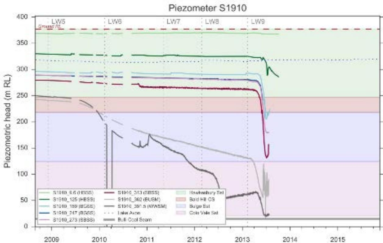
**Figure 39.** Response of the piezometers in bore DDH105/S1910 to the passage of Longwall 9
