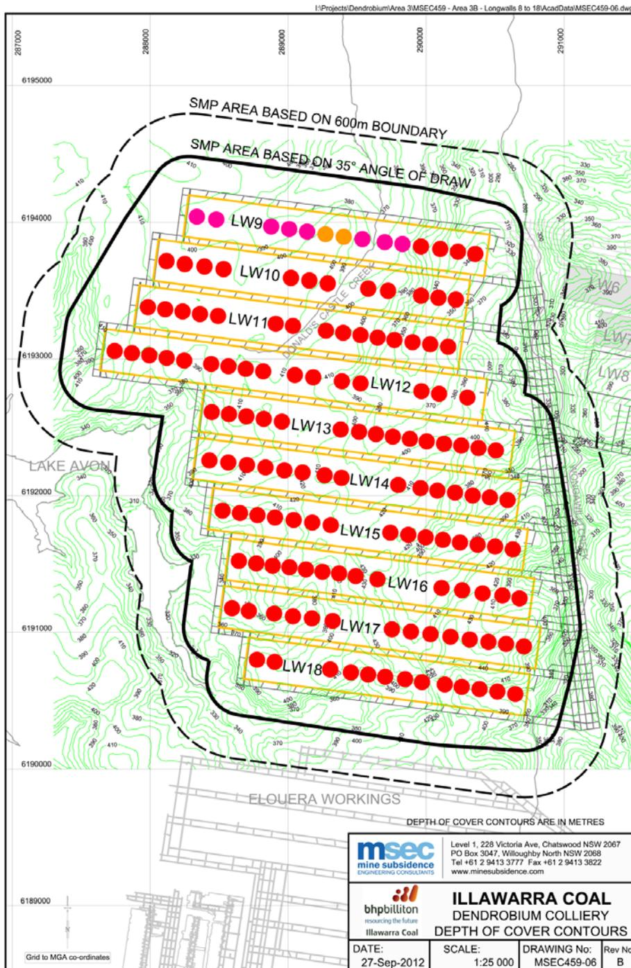
**Figure 21.** Depiction of the height of the drainage zone for 4.6m high extractions in Area 3B
