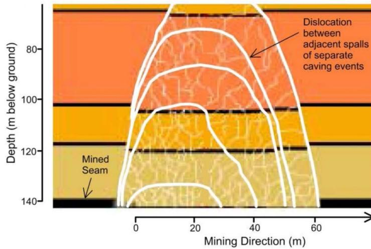
**Figure 4(a).** Development of the drainage zone as a longwall extraction progresses.[2]
