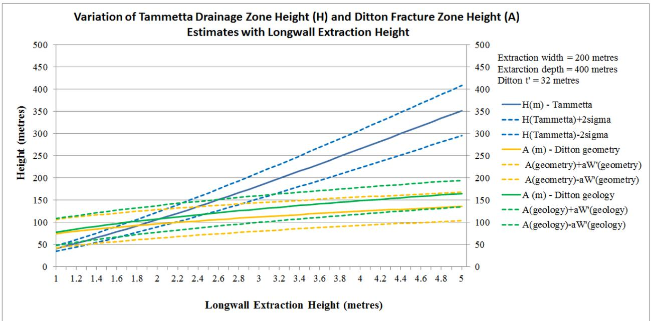
Figure 7. Tammetta and Ditton equation height estimate variations with extraction height.
