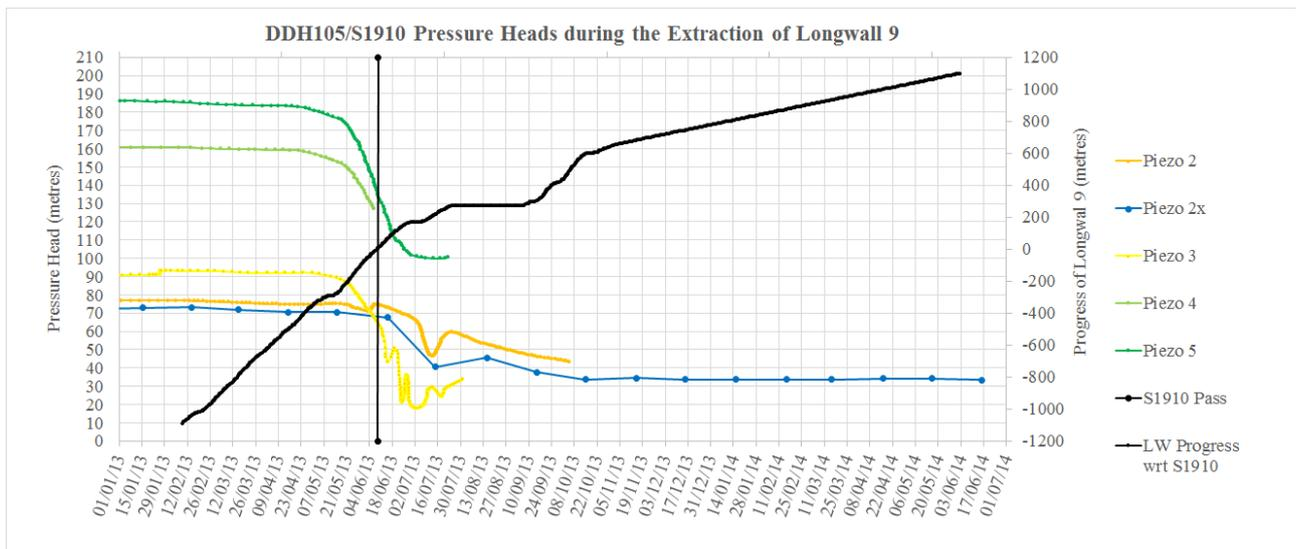
**Figure 38.** Pressure head hydrographs from off-panel bore DDH105/1910 during the extraction of Longwall 9.
