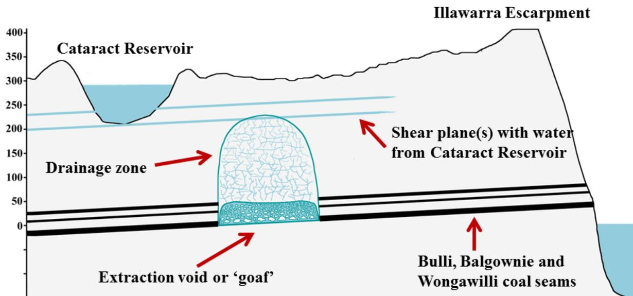
**Figure 58.** Depiction of the drainage zone formed above double seam extractions at the Russell Vale colliery intersecting a water bearing shear plane.
