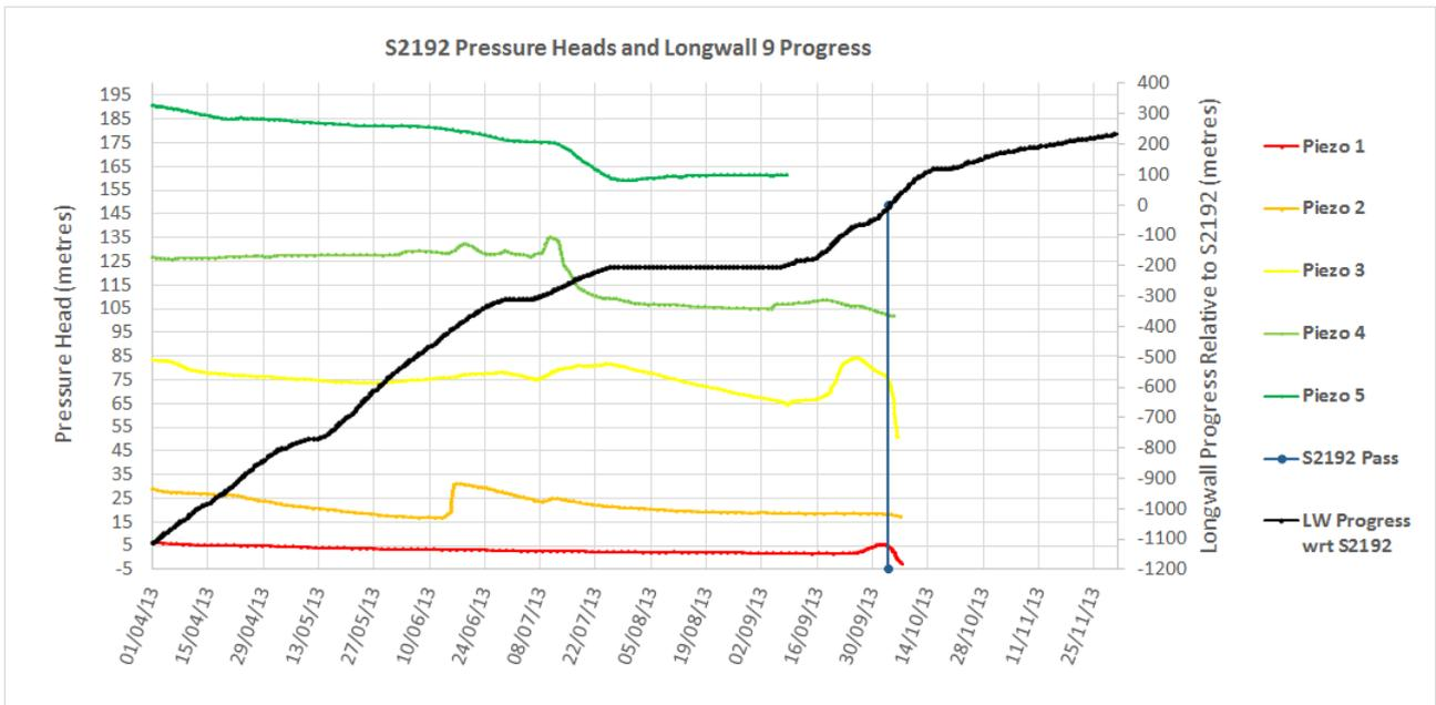
**Figure 43.** Pressure heads from S2192 piezometers 1 to 6 and Longwall 9 progress
