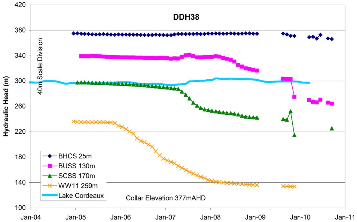
**Figure 29.** DDH38 piezometer hydrographs from the November 1012 Coffey data analysis report.[62]
