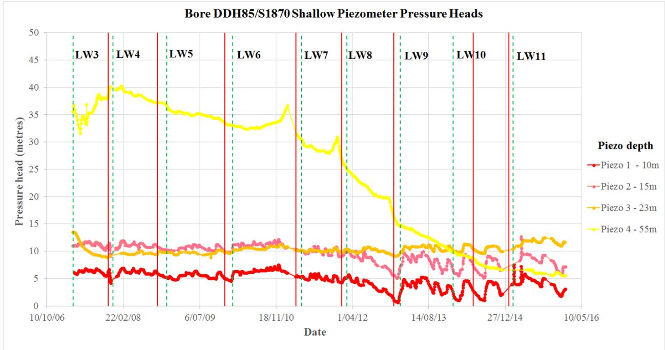
**Figure 36.** Pressure heads recorded by Piezometers 1 to 4 in TARP bore DDDH85/S1870.
