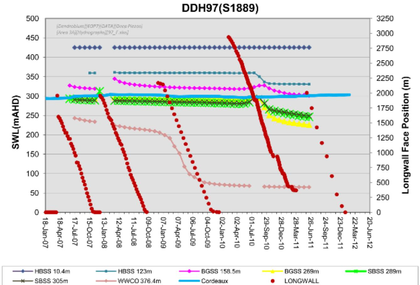
**Figure 33.** Hydrographs from piezometer bore DDH97/S1889
