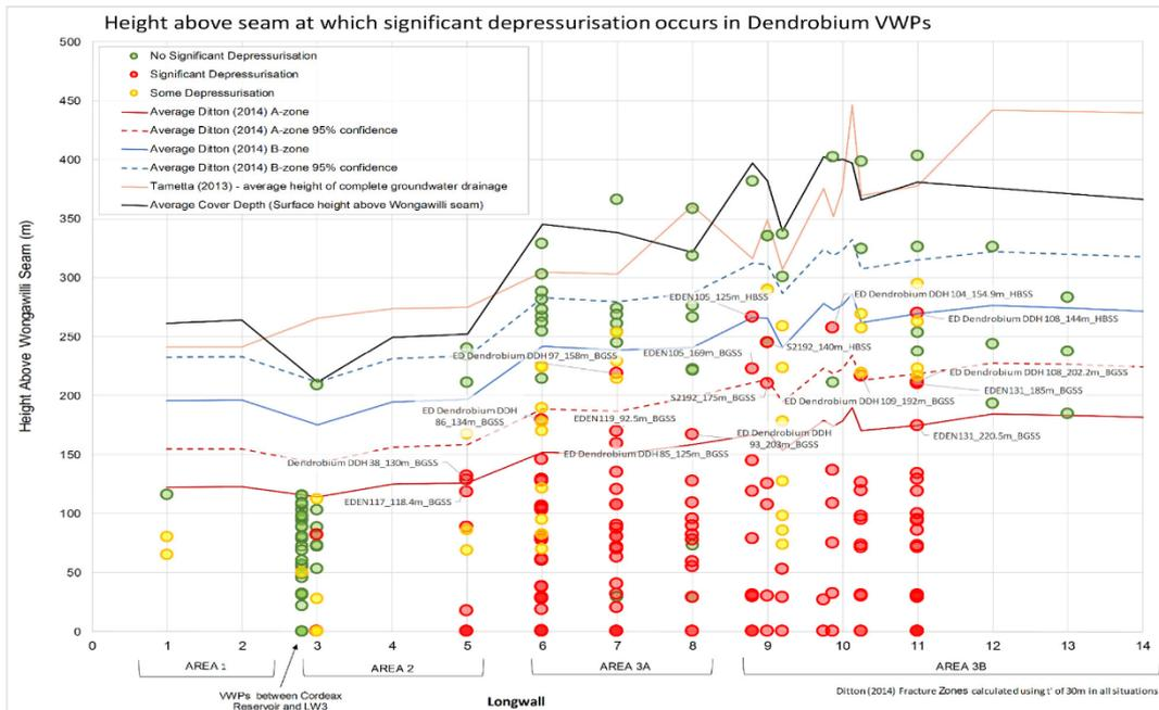
Figure 21 Summary of Groundwater Depressurisation and Estimated Height of Connected Fracturing
