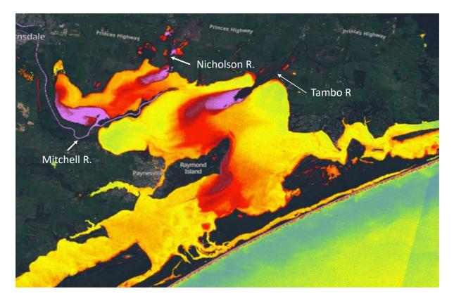
**Figure 2**: False colour Sentinel2 satellite images of Lake King (a Gippsland Lake) processed using the Se2WaQ script set to highlight suspended sediments. Yellow is the lowest suspended sediment concentration - purple is the highest. The image shows all the sediments are being delivered from the three rivers that flow into the lake.
