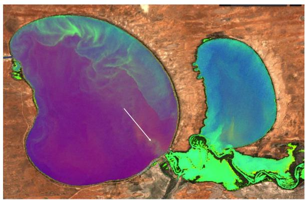
**Figure 6:** False colour Sentinel 2 satellite image of the whole of Lake Pamamaroo and Lake Tandure and the lower portion of Lake Wetherell taken on March 14 and processed with the APA script. Green and yellow represent levels of high algal density. Purple is high concentrations of suspended sediments. The arrow represents a potential flow path as water was being released from Lake Pamamaroo.
