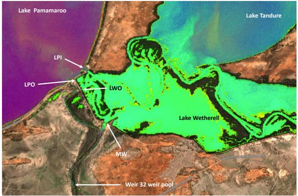
**Figure 2**: False colour Sentinel 2 satellite image of the bottom end of Lake Wetherell and the top end of weir 32 weir pool taken on March 14 processed with the APA script (Péliova et al, undated). Algal biomass is shown in green. MW = Main Weir; LPI = Lake Pamamaroo inlet; LPO = Lake Pamamaroo outlet; LWO = Lake Wetherell outlet.
