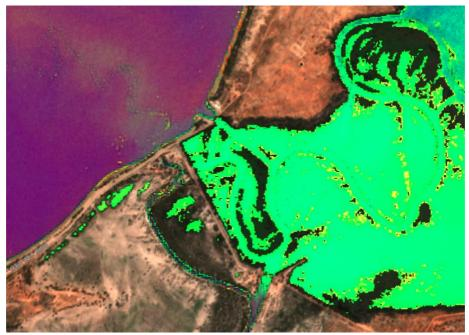
**Figure 4:** False colour Sentinel 2 satellite image of the same region as Figure 3, taken on March 14 and processed with the APA script. Green and yellow represent levels of high algal density. Purple is high concentrations of suspended sediments
