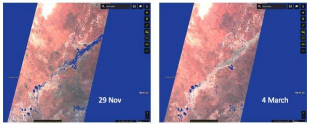
**Figure 1**: False colour Sentinel2 satellite imagery of the Darling River floodplain processed with the Water in Wetlands script (Willm et al, undated) highlighting water in blue.
