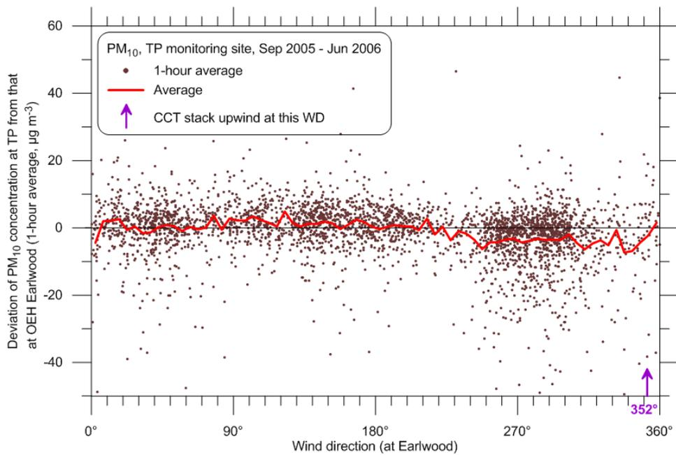
Figure 56 PM<sub>10</sub> deviations at TP vs wind direction for 2005-2006
