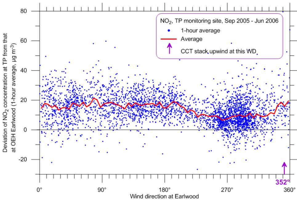
Figure 44 NO<sub>2</sub> deviations at TP vs wind direction for 2005-2006
