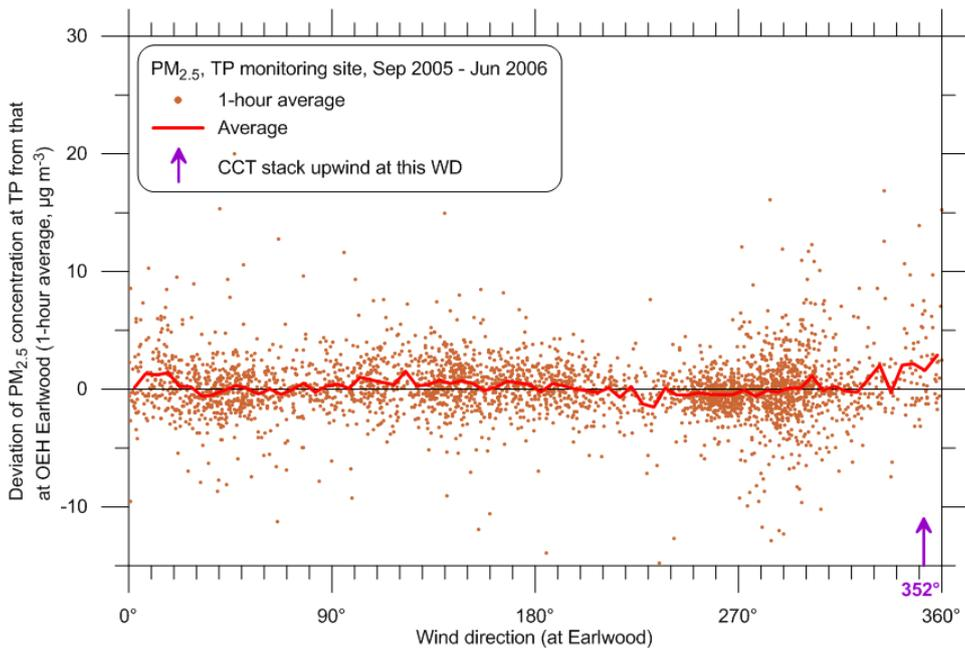
Figure 52 PM<sub>2.5</sub> deviations at TP vs wind direction for 2005-2006
