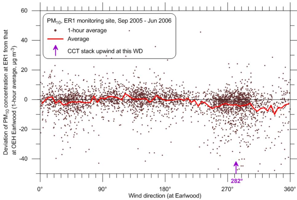
Figure 53 PM<sub>10</sub> deviations at ER1 vs wind direction for 2005-2006
