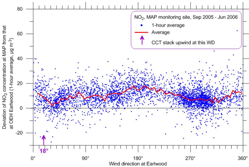
Figure 43 NO<sub>2</sub> deviations at MAP vs wind direction for 2005-2006
