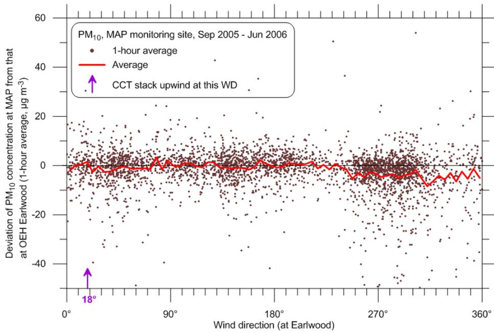
Figure 55 PM<sub>10</sub> deviations at MAP vs wind direction for 2005-2006
