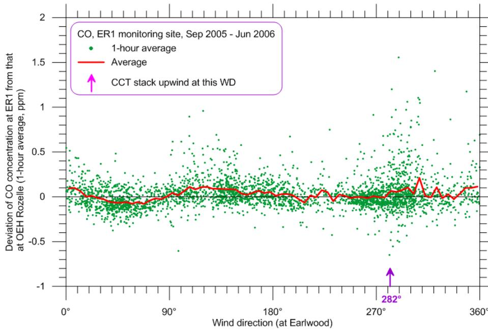
Figure 45 CO deviations at ER1 vs wind direction for 2005-2006
