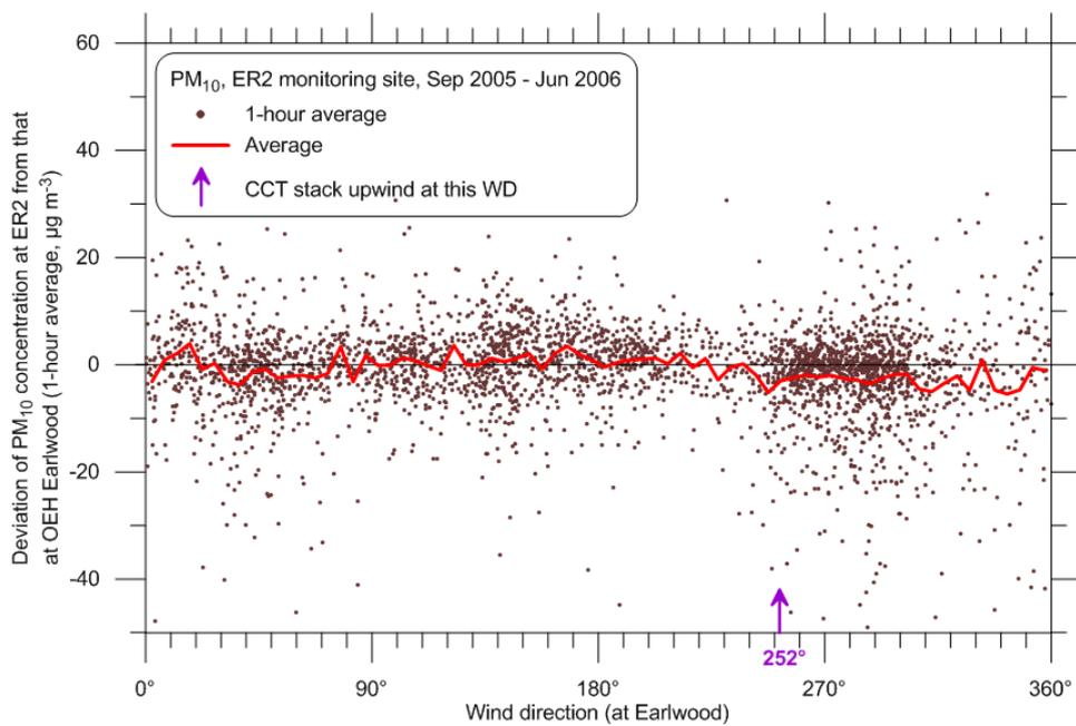
Figure 54 PM<sub>10</sub> deviations at ER2 vs wind direction for 2005-2006
