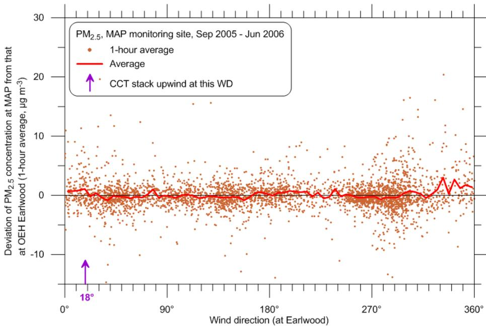
Figure 51 PM<sub>2.5</sub> deviations at MAP vs wind direction for 2005-2006
