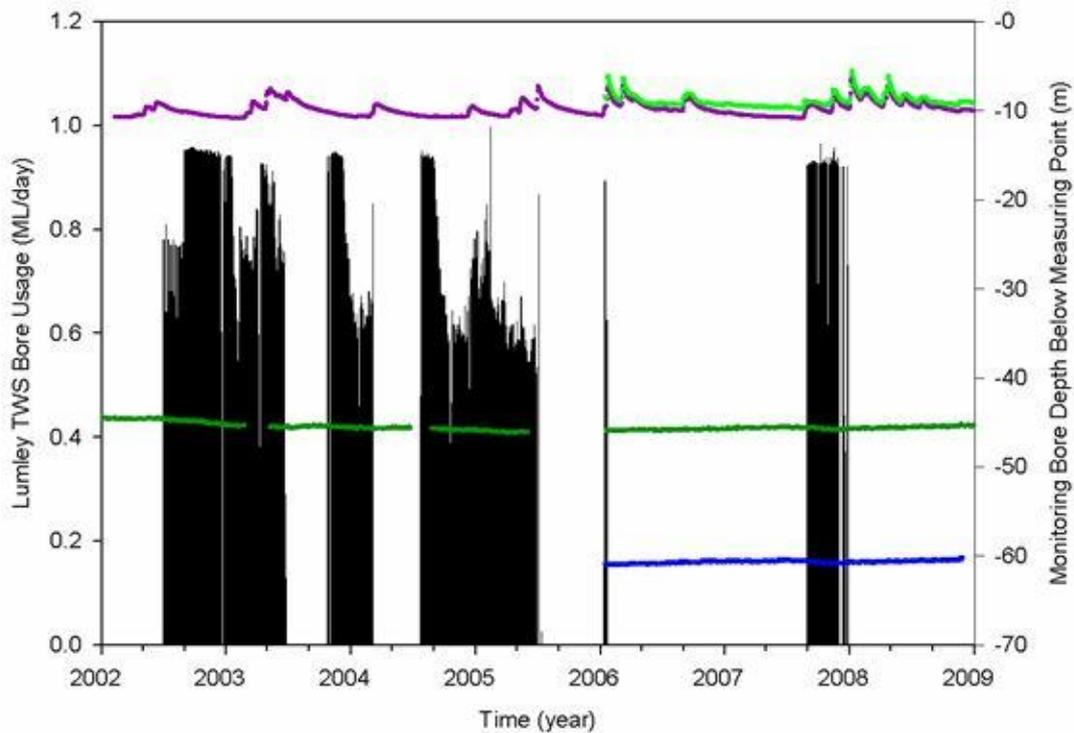
**Figure 37:** Lumley Park TWS bore usage (black columns) and water level and/or pressure observed at DPIE monitoring bores GW081006 (shallow) and GW081005 (deeper) from 2002 to 2009.
