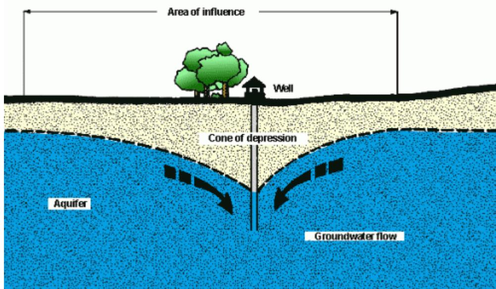
**Figure 21: Area of influence and cone of depression in the aquifer due to groundwater pumping**
