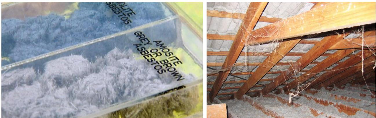
**Figure 3.5: Loose fill type asbestos – friable** <sup>5</sup>
