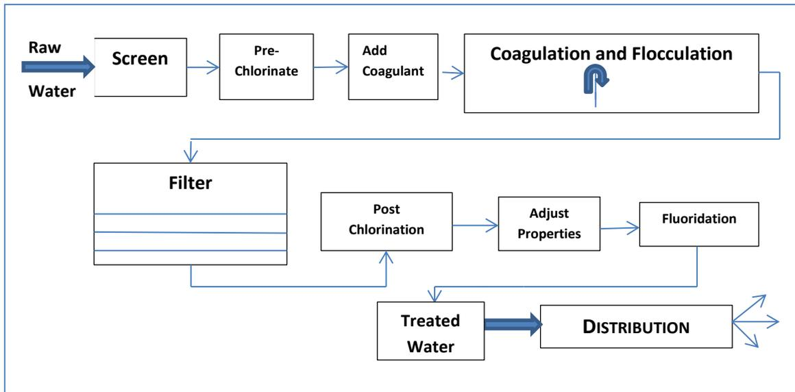
**Figure 3: Water Filtration Plant**
