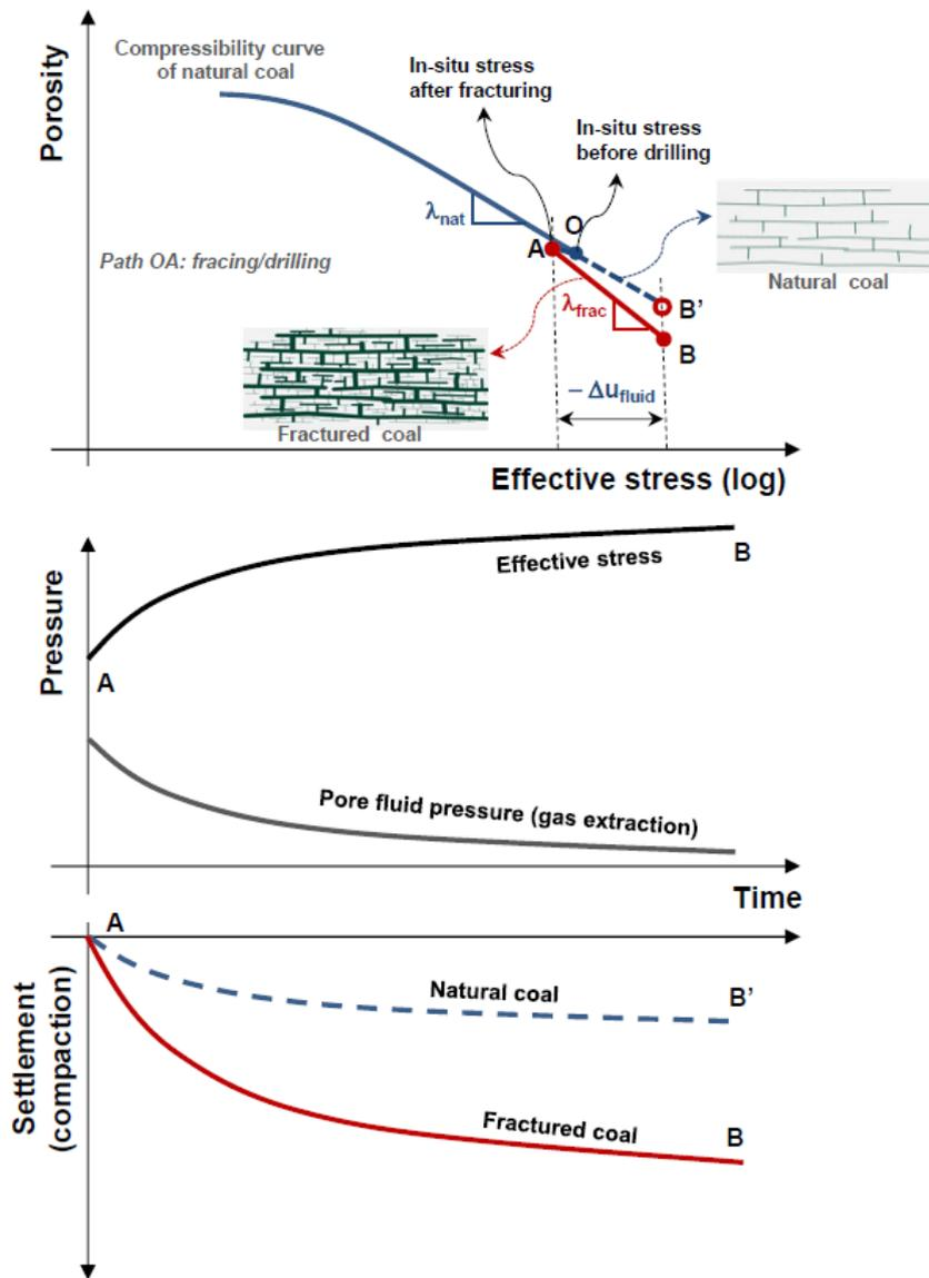
Figure 20. Schematic view of the coal seam compaction
