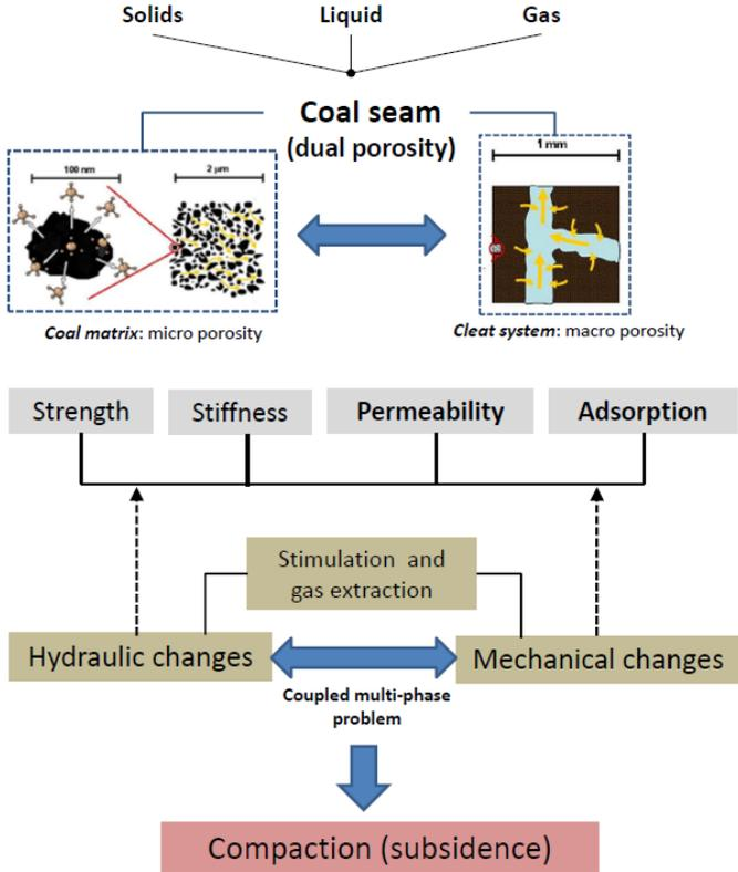
Figure 24. Schematic representation of subsidence in CSG extraction
