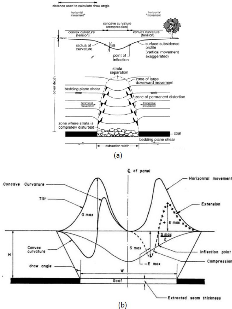
Figure 8. Subsidence in longwall mining. (a) Subsidence model (Hall & Barclay, 2000). (b) Development of vertical and horizontal displacements
