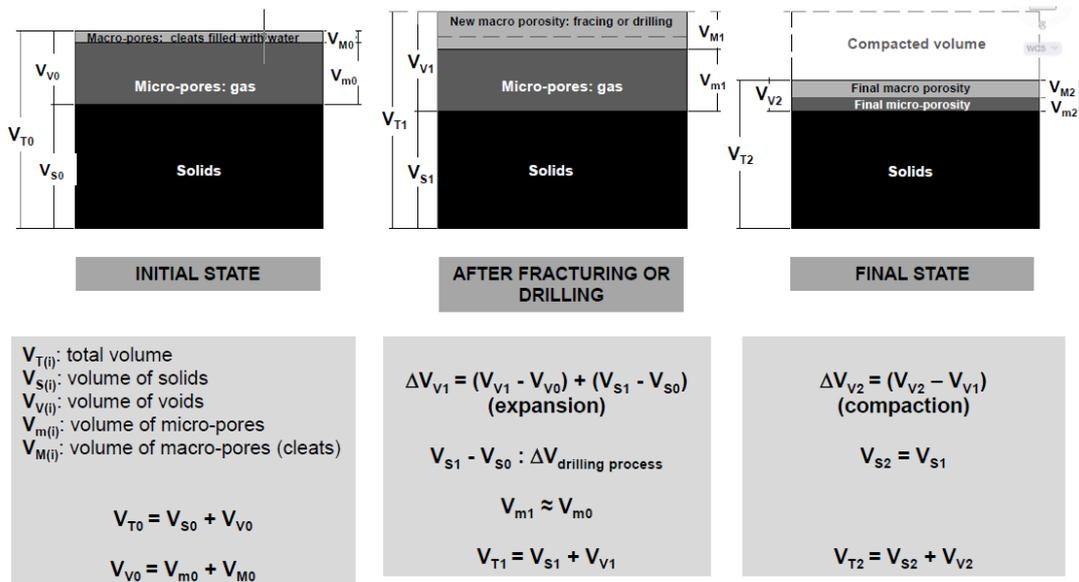
Figure 19. Phase diagrams for the coal seam compaction
