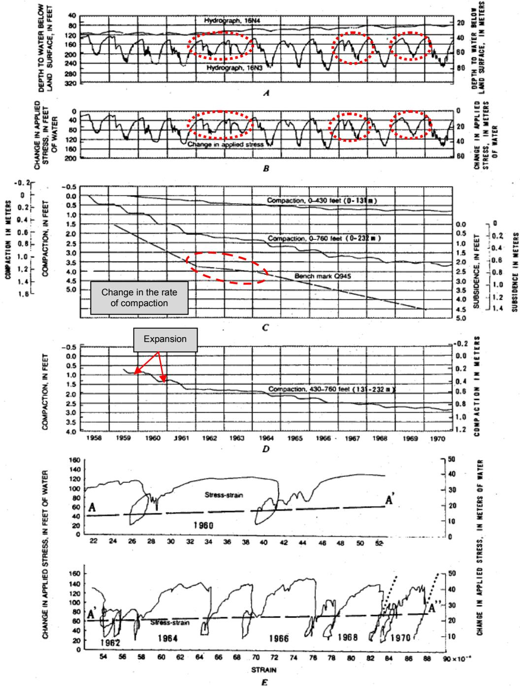
Figure 11. Ground water extraction in San Joaquin Valley. (a) Hydrographs. (b) Changes in applied stresses. (c) Compaction in different levels. (d) Compaction in 131-232m depth interval. (e) Stress changes vs strain (from Poland et al, 1975)
