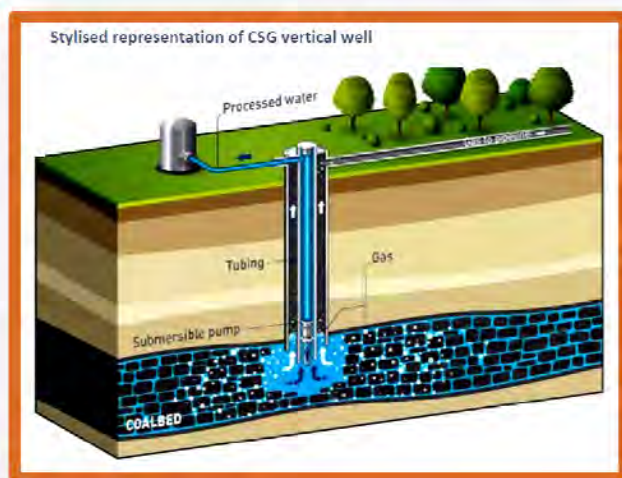
Figure 1.7 (left): A "producing" CSG vertical well (Rutovitz et al., 2011, p.22)
